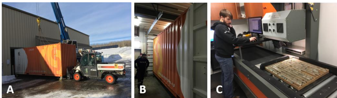
Figure 2A. Fully Mobile Corescan laboratory being delivered to the MnDNR Core Library; 2B. Placement in the interior of the Core Library and 2C. Internal view of the Corescan laboratory with Corebox translation table, imaging system and computing infrastructure.
