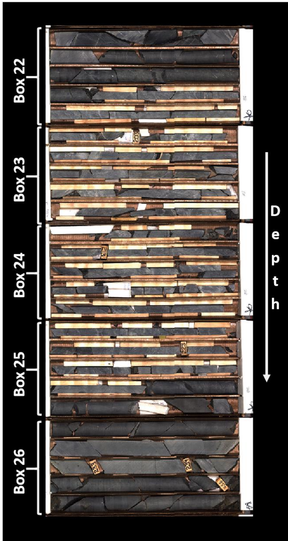
Figure 7. Corescan RGB Digital photography displayed in 'Stacked-by-section' format where imaged core boxes are 'stacked' digitally with depth; this imagery taken from a high gold grade zone in the International Falls Greenstone Gold Focus Area (JA0429), drill hole TC36-1 (193'-202').
