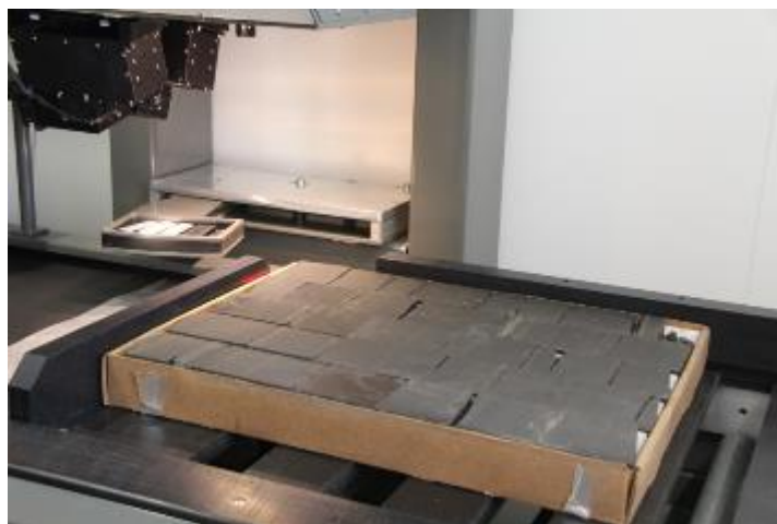
Figure 4. Automated radiometric and wavelength calibration using NIST Spectralon standards prior to scanning of each row of core.
