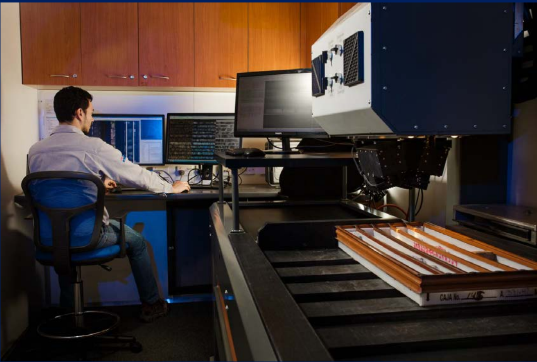
Imaging devices in the Corescan mobile lab include a digital RGB camera (50mm spatial resolution), a 3D Core Surface Profiler for geotechnical logging (~20mm vertical resolution), and VNIR, SWIR-A, and SWIR-B Spectrometers (~4mm spectral resolution)
