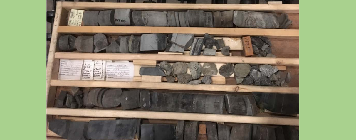
Drill core was either scanned within its storage box or transferred to wood trays as shown. This tray also shows how different types of material was staged for scans.
