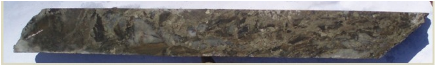
Drill core from the Bigfork Exploration Area. Gold-bearing iron formation with 5.3 gpt/5 ft. (Photo courtesy of Vermillion Gold LLC).
