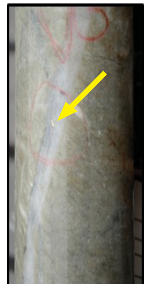
Visible gold grain in a Virginia Horn quartz-feldspar porphyry drill core that has 77.9 gpt/2.3 ft. Photo courtesy of Vermillion Gold LLC
