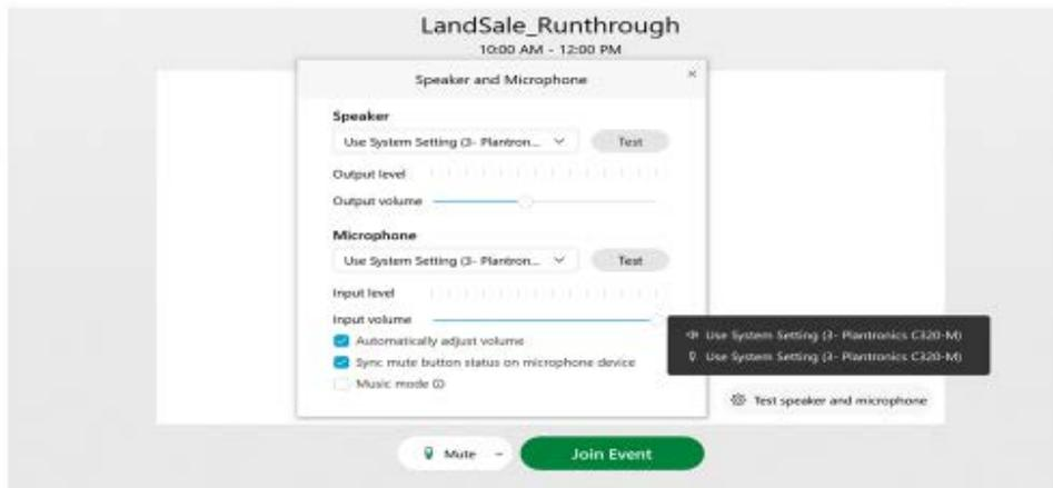
Set equipment shows in the black box and in the drop-down boxes for speaker and microphone. Please Test.
