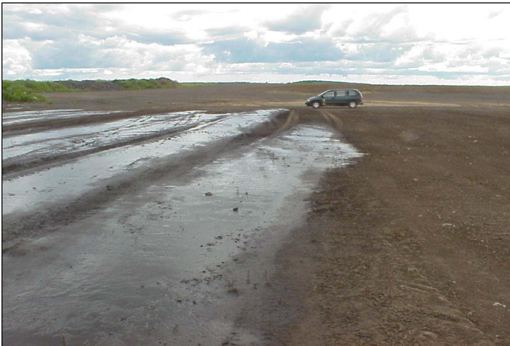
Figure 20. Aurora liquid biosolids landspreading site at Cliffs Erie surface stockpile one hour after application. This was a bare, one-acre test site where seed was added to the biosolids before spreading.
