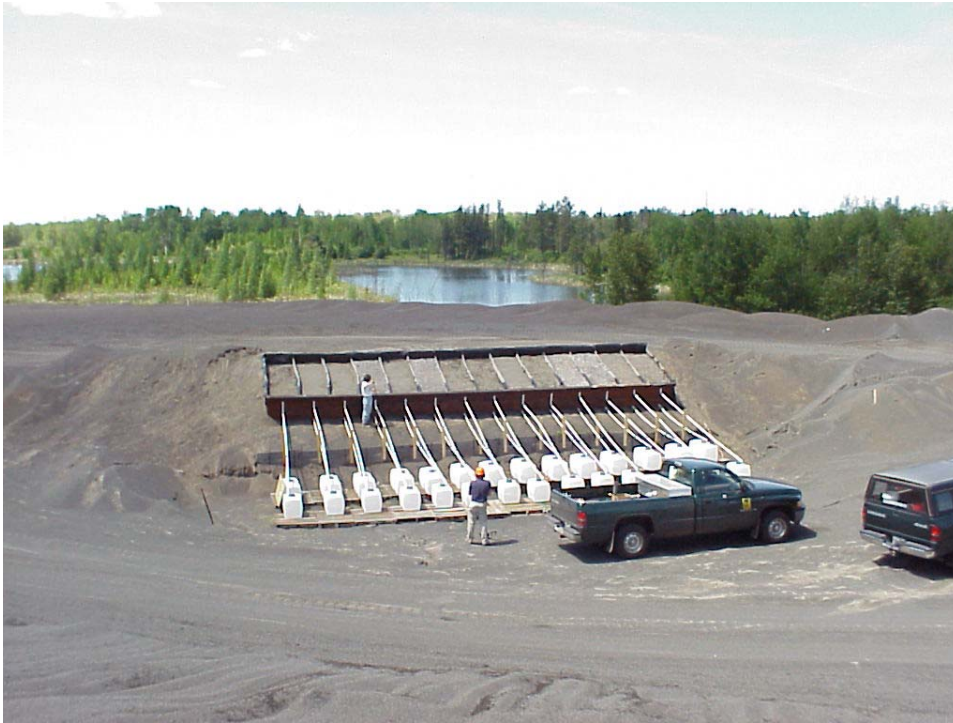
Figure 5. Biosolids bin plots at United Tac. White barrels are to collect water samples for water quality testing.
