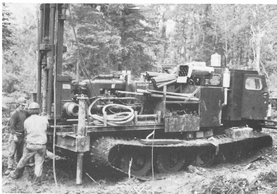
PHOTO B. CRAWLER-MOUNTED CME 55 RIG ON DRILL HOLE CASA-3056.
