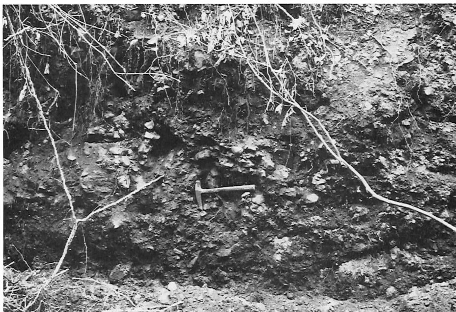
PHOTO B. EXPOSURE OF GRAVELLY SAND IN 5-FOOT HIGH ROAD CUT, ON WEST SLOPE OF EAST RIDGE ABOUT 1000 FEET SOUTH OF EAST ABUT- MENT CONTACT OF DAM NO. 1. GEOLOGIST'S PICK GIVES SCALE.
