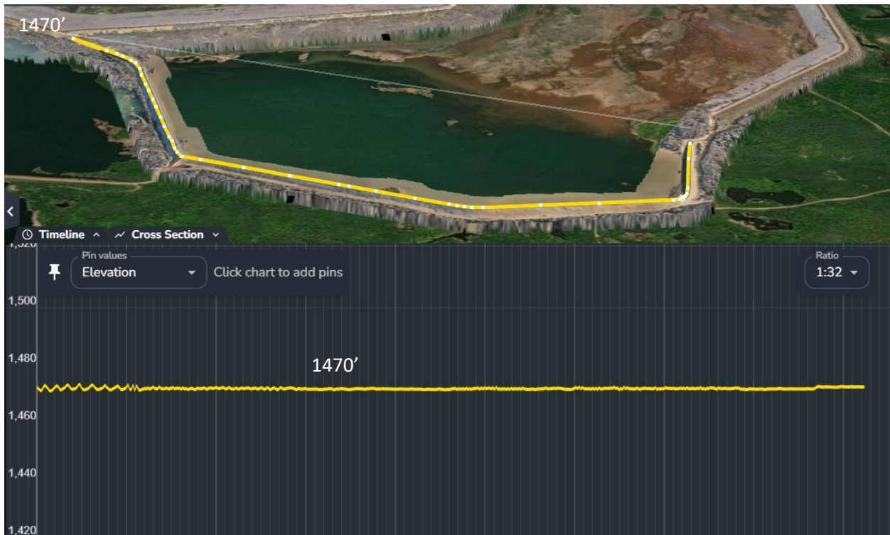
Figure 4: Stage 2 Exterior Water Dam Crest Elevations
