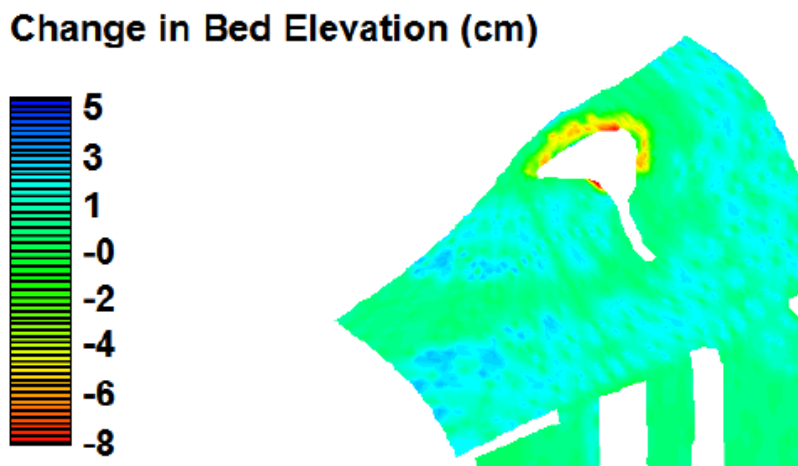
Figure 4-5 Color contoured plot of the change in bed elevation in Block 10 for the shoals design.
