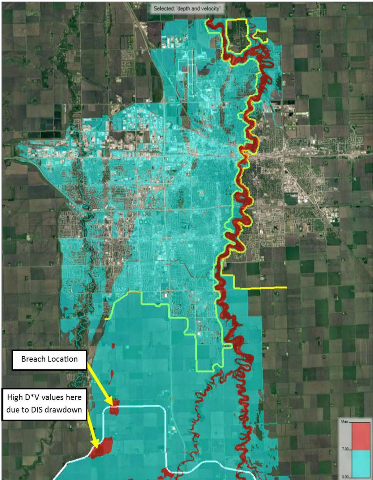
**Figure 10. Proposed Conditions Maximum D\*V for 90,000 cfs Event after Dam Breach at Location 1**
