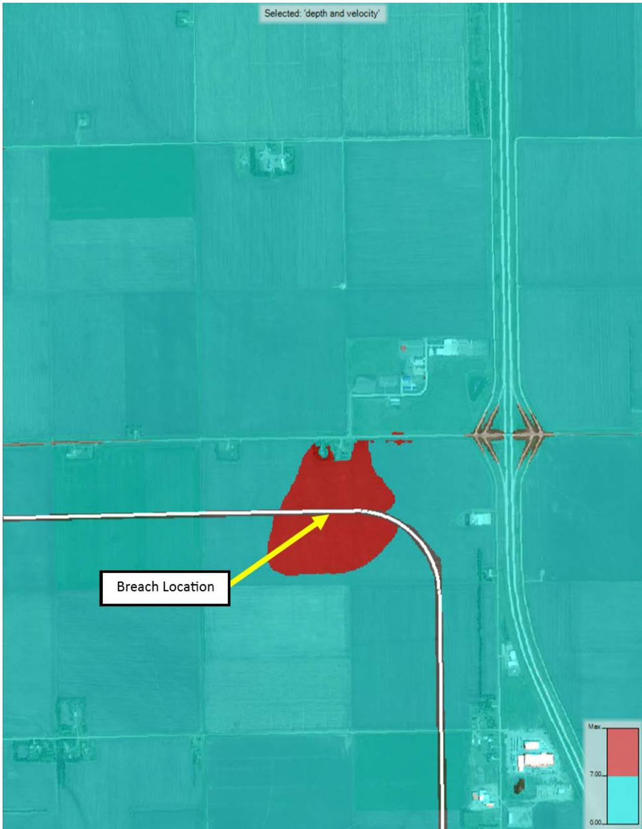
**Figure 14. Proposed Conditions Near-Vicinity Maximum  $D*V$  for 90,000 cfs Event after Dam Breach at Location 2**
