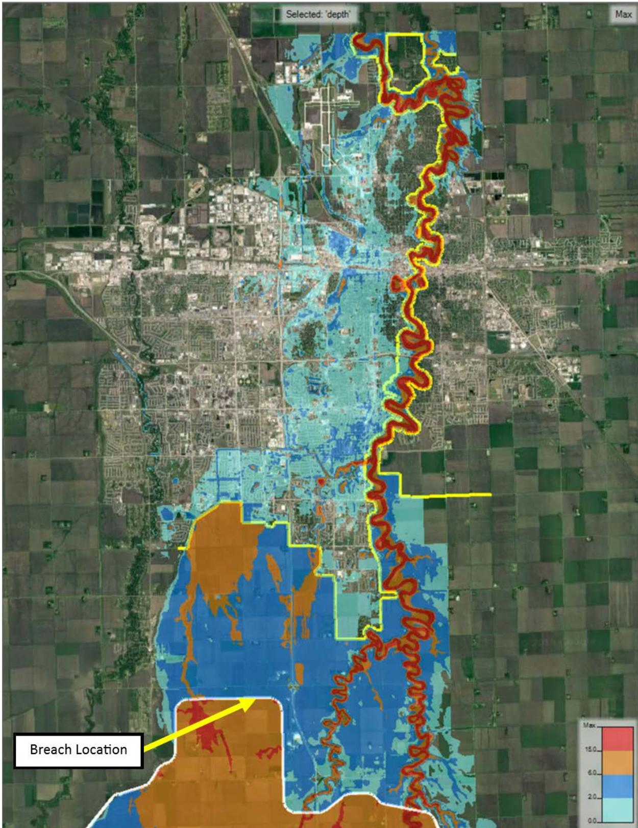
**Figure 12. Proposed Conditions Maximum Flow Depths for 90,000 cfs Event after Dam Breach at Location 2**
