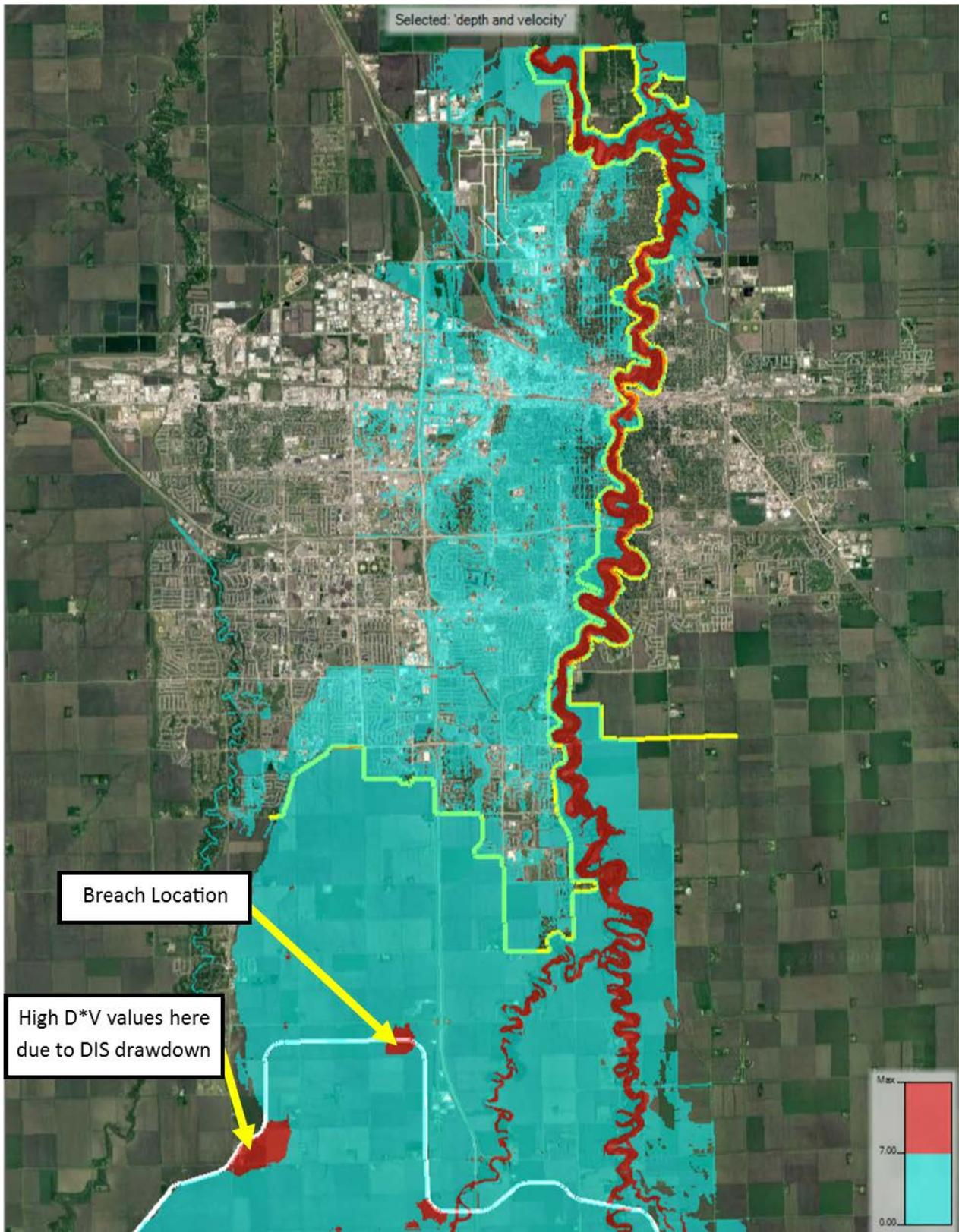
**Figure 13. Proposed Conditions Maximum D\*V for 90,000 cfs Event after Dam Breach at Location 2**
