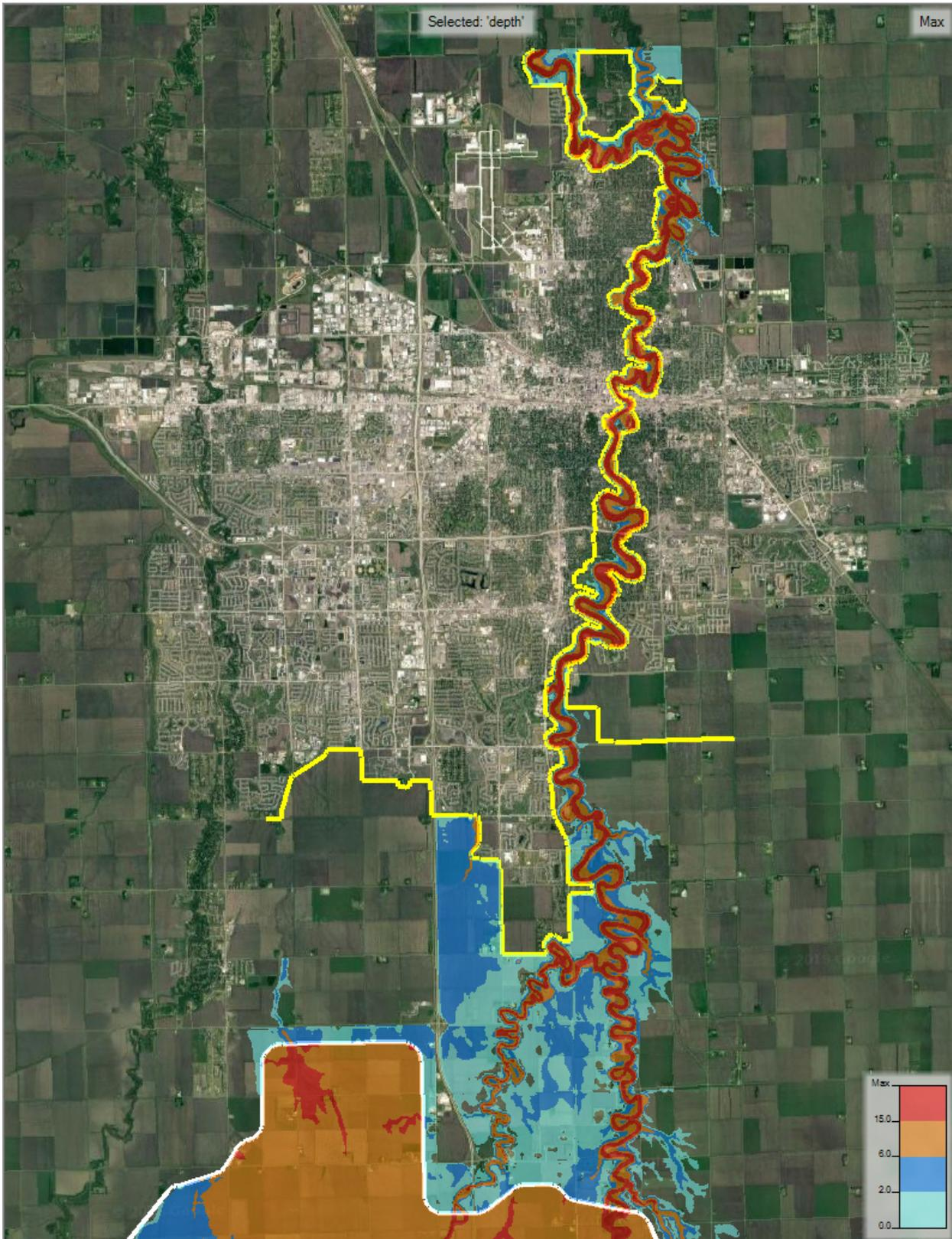
**Figure 8. Proposed Conditions Maximum Flow Depths for 90,000 cfs Event (No Dam or Levee Breach)**
