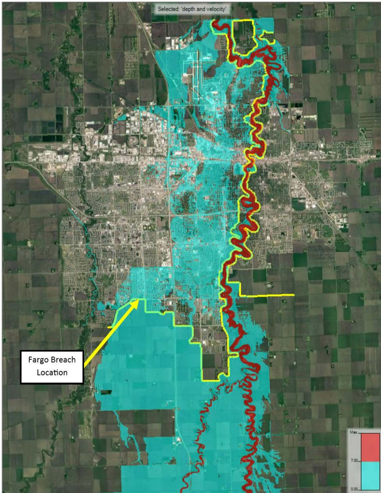
**Figure 31. Existing Conditions Maximum D\*V for 1% ACE Event after Fargo Levee Breach**
