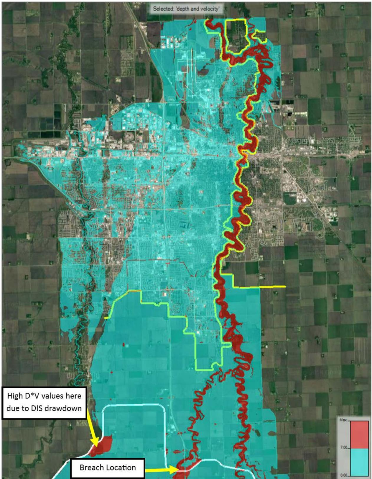
**Figure 19. Proposed Conditions Maximum D\*V for 90,000 cfs Event after Dam Breach at WRRS**
