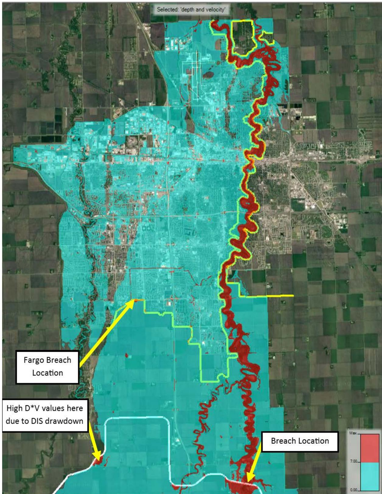
**Figure 37. Proposed Conditions Maximum D\*V for 1% ACE Event after Dam Breach at RRS and Fargo Levee**
