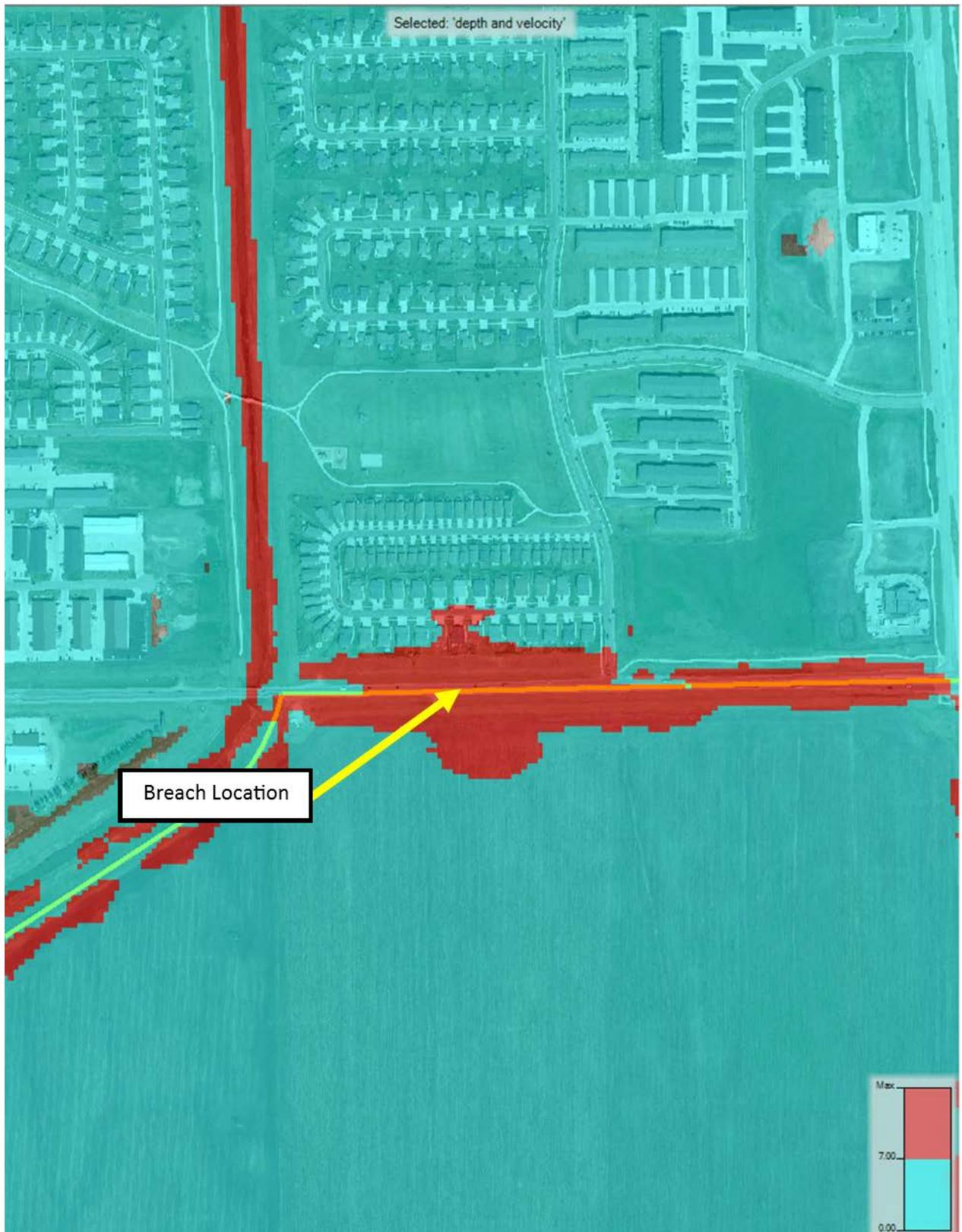
**Figure 38. Proposed Conditions Near-Vicinity Maximum D\*V for 1% ACE Event after Dam Breach at RRS and Fargo Levee**
