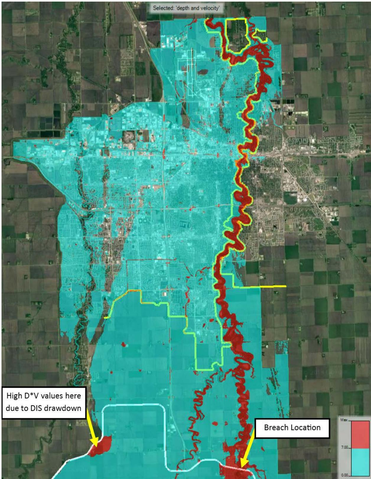
**Figure 22. Proposed Conditions Maximum D\*V for 90,000 cfs Event after Dam Breach at RRS**
