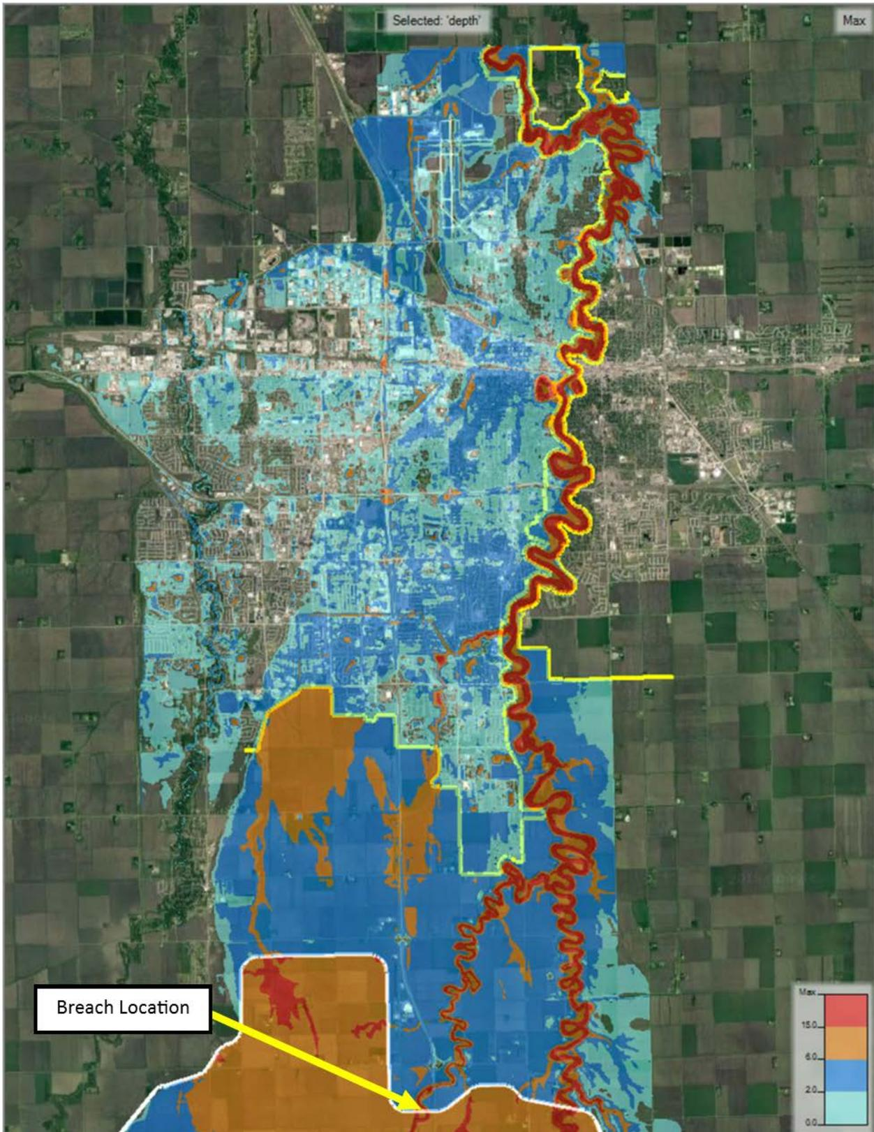
**Figure 18. Proposed Conditions Maximum Flow Depths for 90,000 cfs Event after Dam Breach at WRRS**
