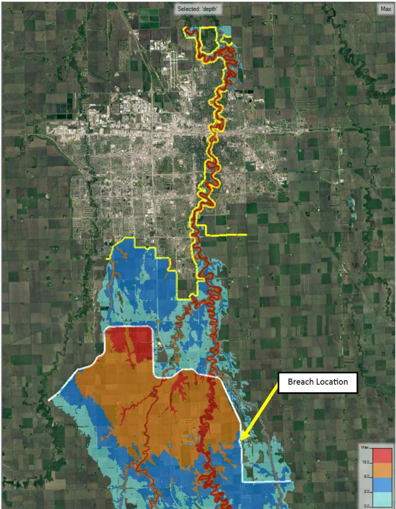
**Figure 15. Proposed Conditions Maximum Flow Depths for 90,000 cfs Event after Dam Breach at Location 3**
