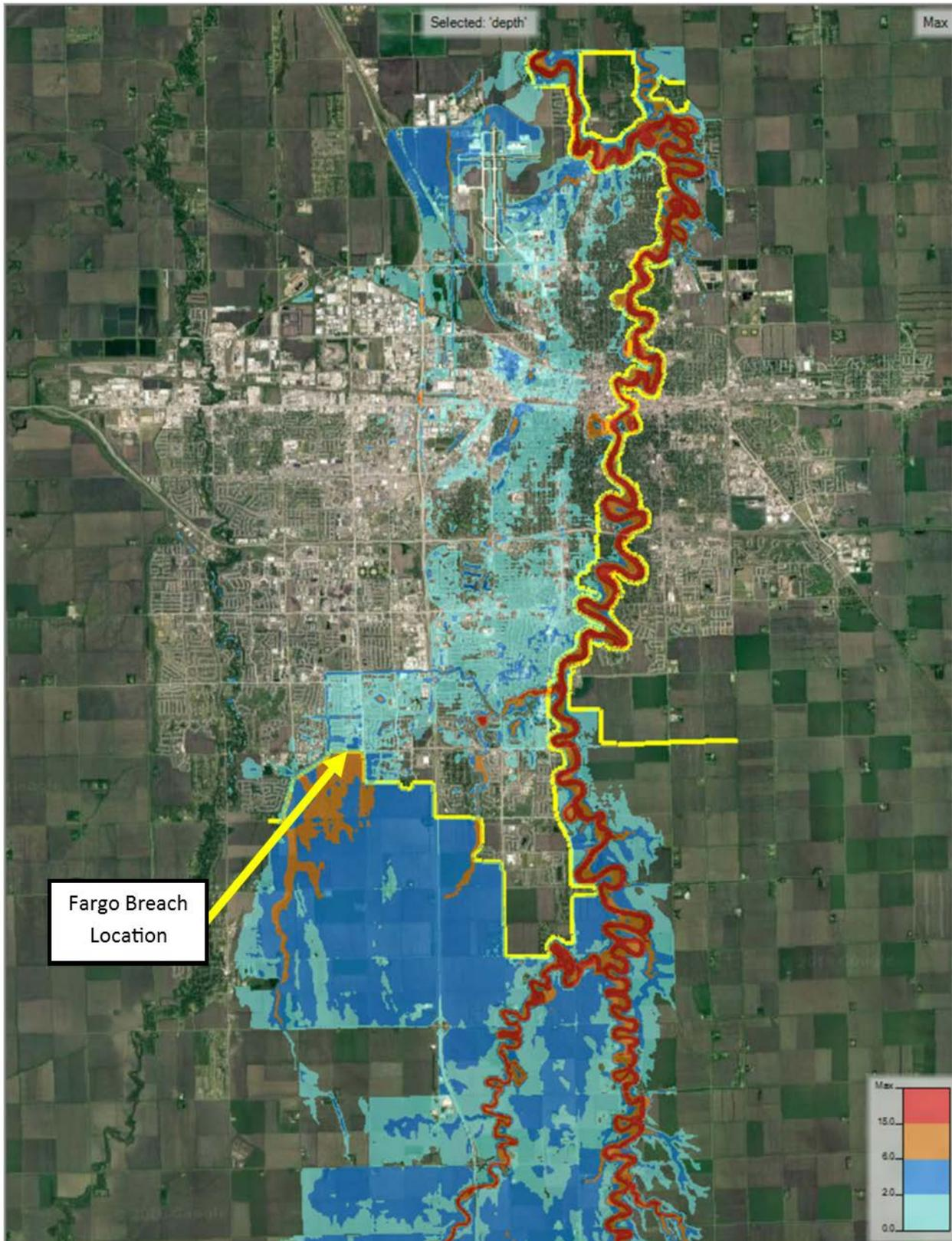
**Figure 30. Existing Conditions Maximum Flow Depths for 1% ACE Event after Fargo Levee Breach**
