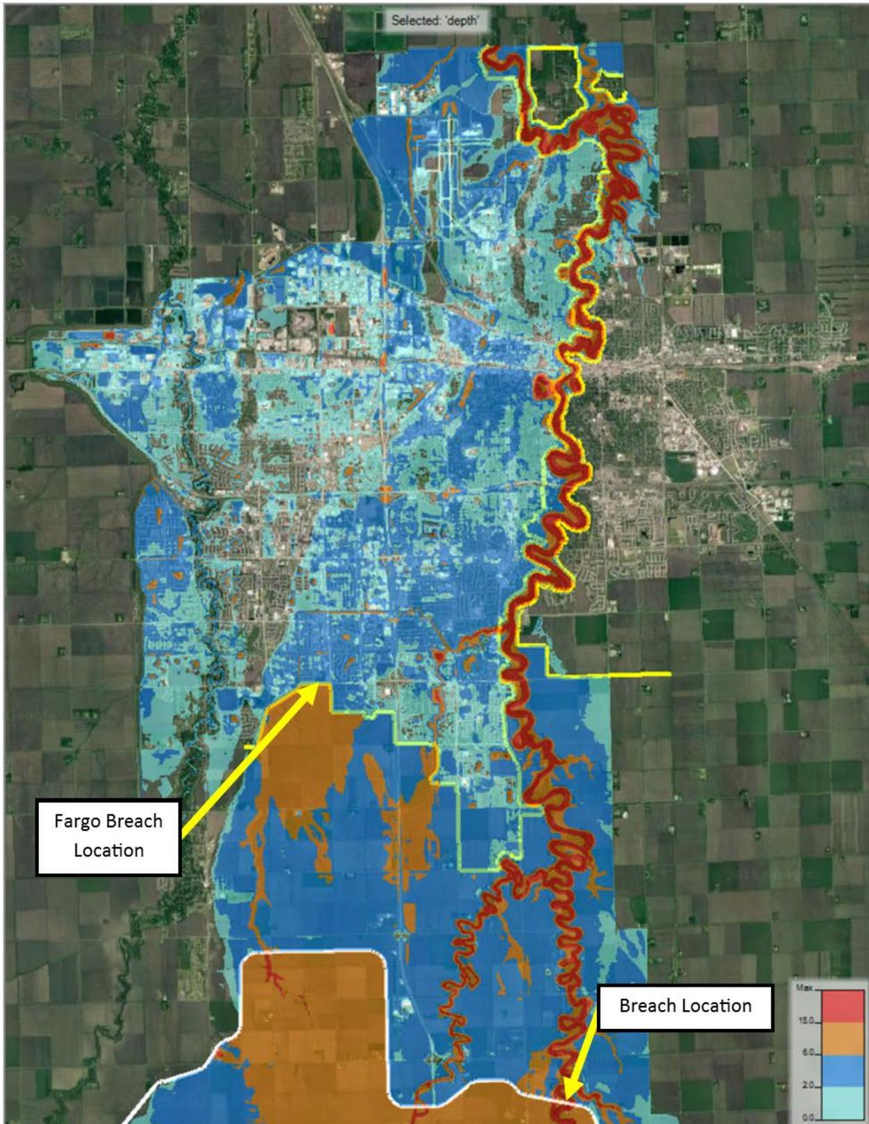
**Figure 36. Proposed Conditions Maximum Flow Depths for 1% ACE Event after Dam Breach at RRS and Fargo Levee**
