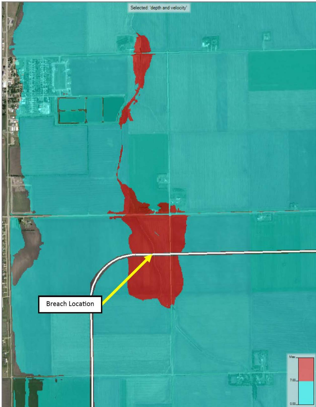
**Figure 11. Proposed Conditions Near-Vicinity Maximum  $D*V$  for 90,000 cfs Event after Dam Breach at Location 1**
