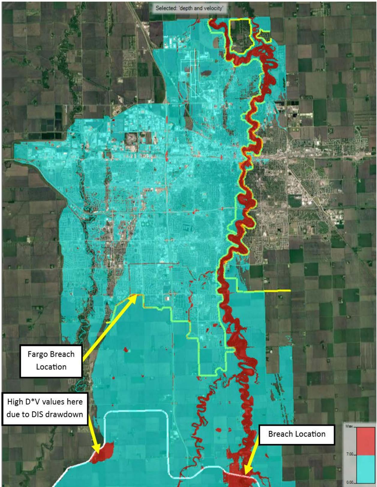
**Figure 25. Proposed Conditions Maximum D\*V for 90,000 cfs Event after Dam Breach at RRS and Fargo Levee**
