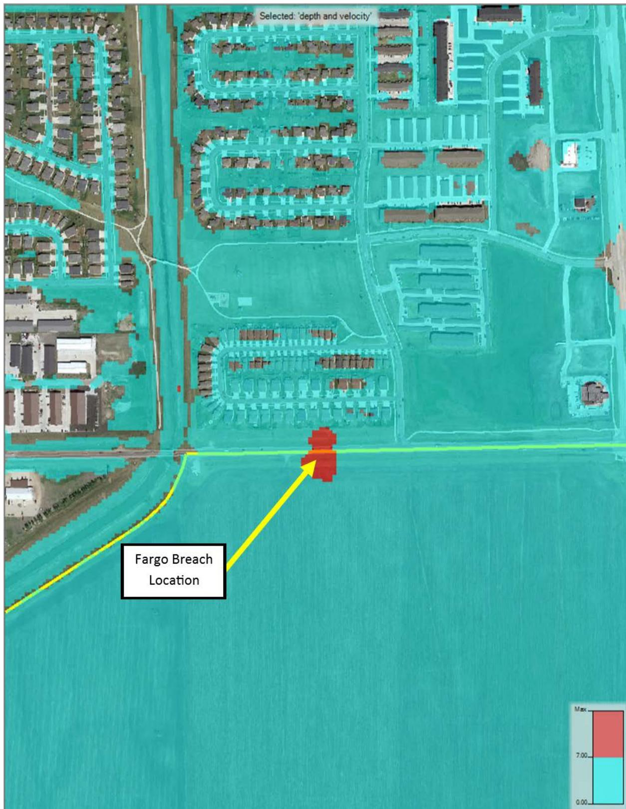
**Figure 32. Existing Conditions Near-Vicinity Maximum D\*V for 1% ACE Event after Fargo Levee Breach**
