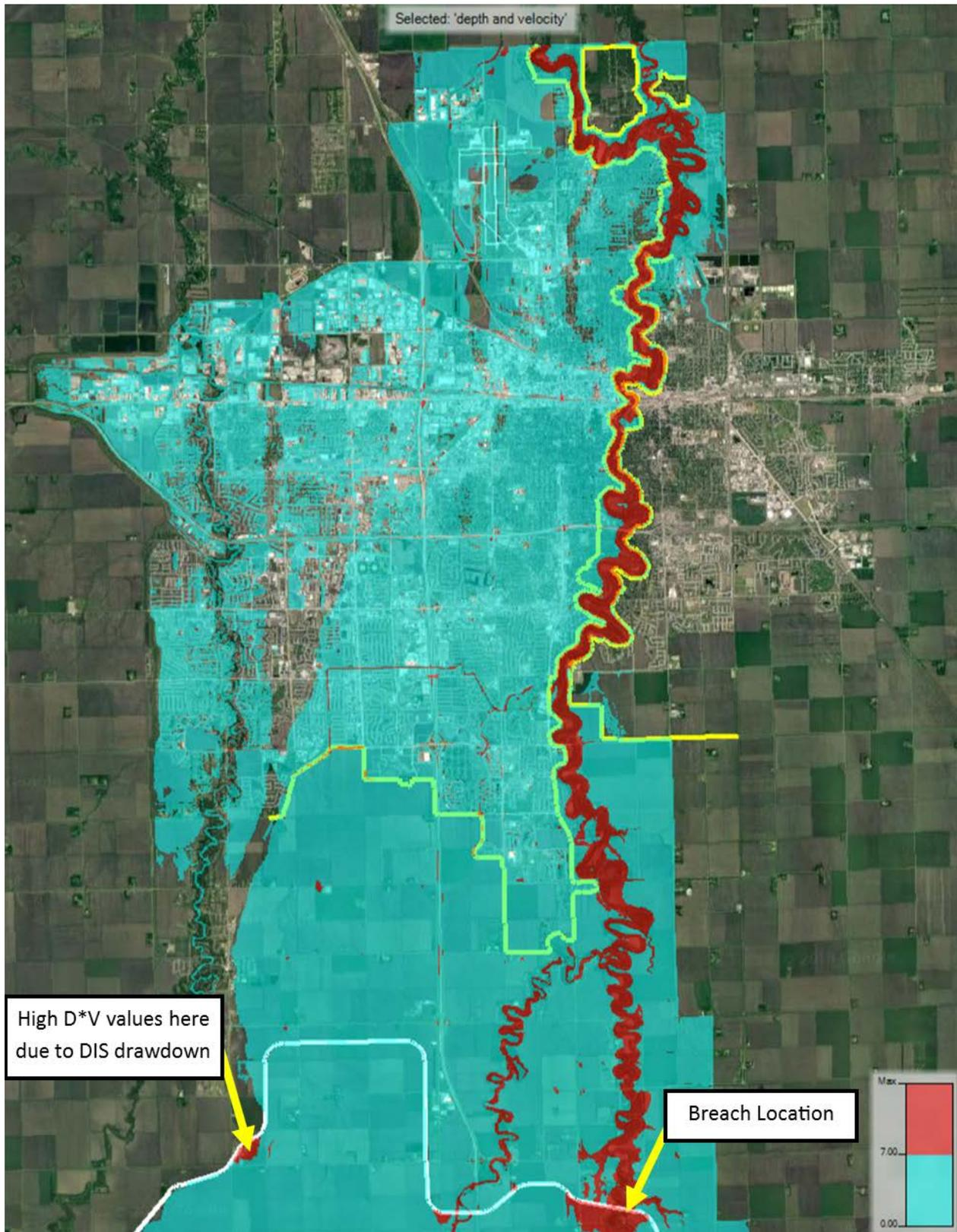
**Figure 34. Proposed Conditions Maximum D\*V for 1% ACE Event after Dam Breach at RRS**
