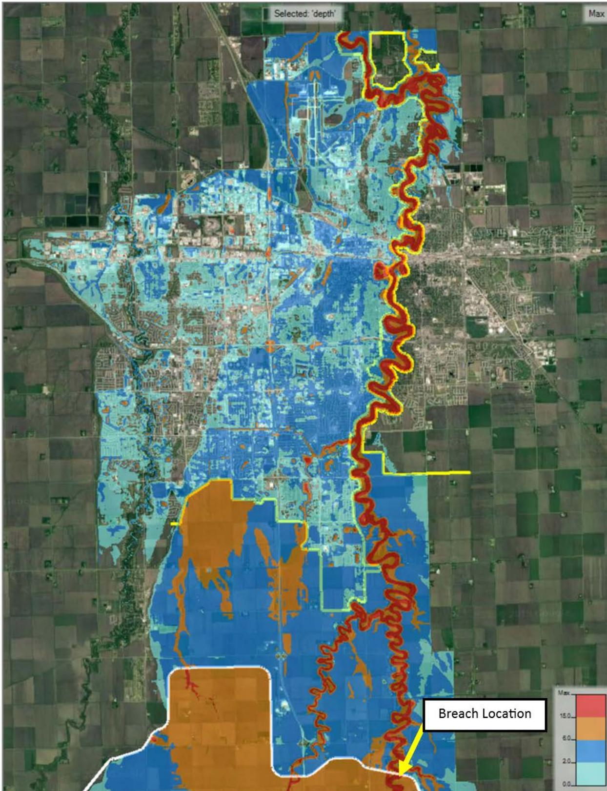
**Figure 33. Proposed Conditions Maximum Flow Depths for 1% ACE Event after Dam Breach at RRS**
