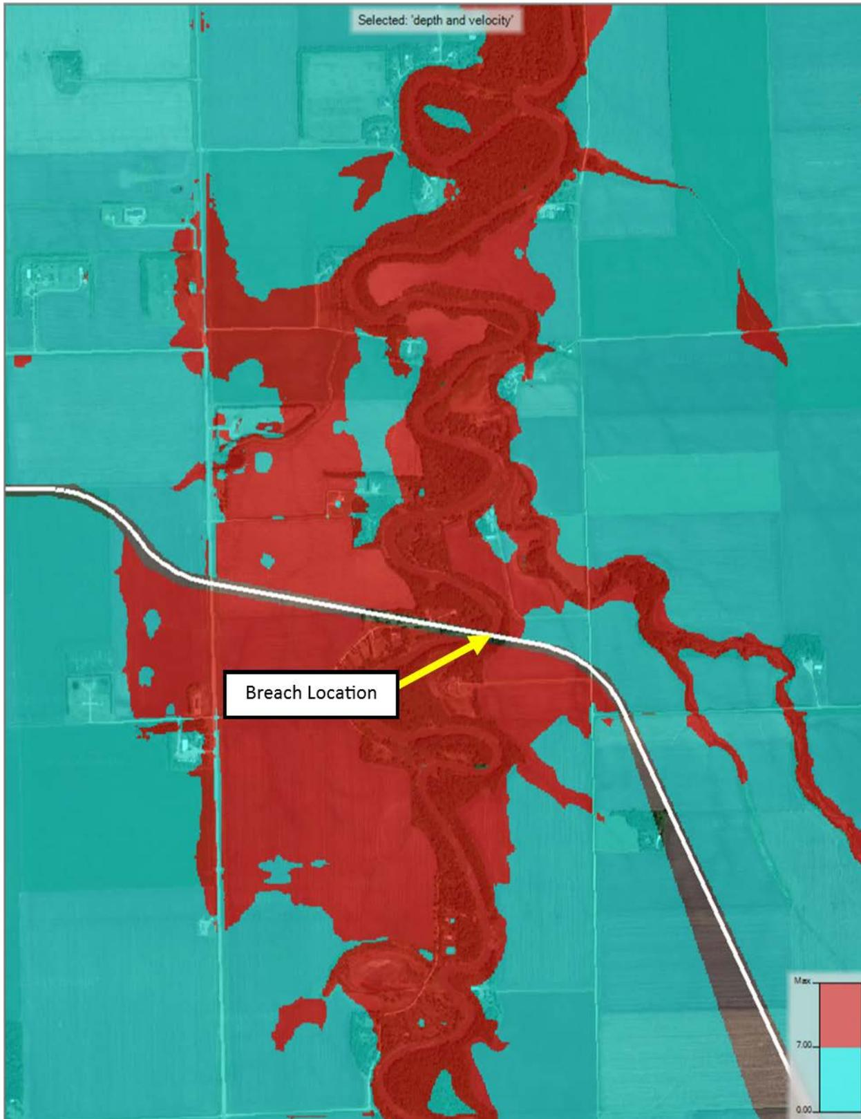
**Figure 23. Proposed Conditions Near-Vicinity Maximum D\*V for 90,000 cfs Event after Dam Breach at RRS**
