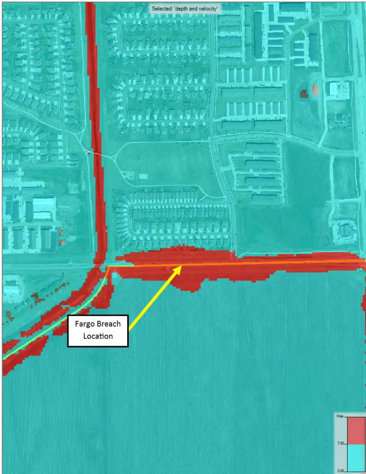
**Figure 26. Proposed Conditions Near-Vicinity Maximum D\*V for 90,000 cfs Event after Dam Breach at RRS and Fargo Levee**
