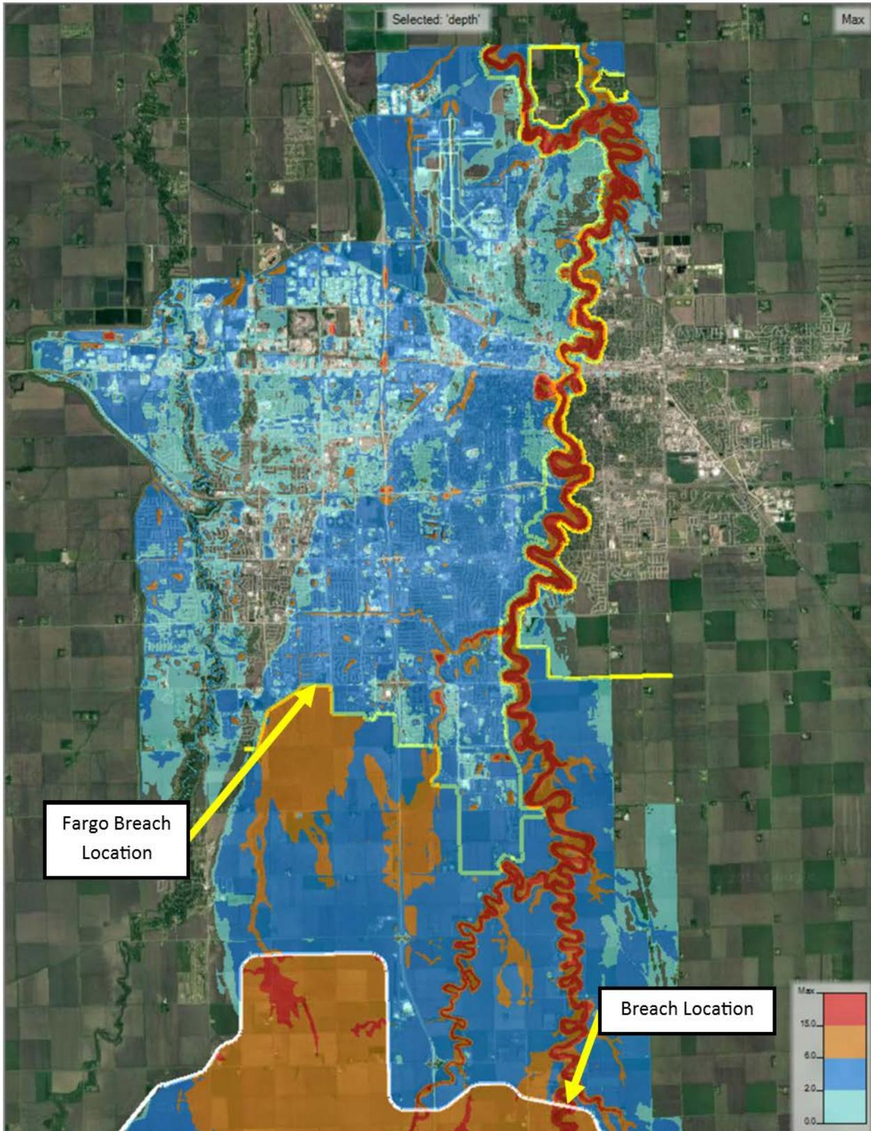
**Figure 24. Proposed Conditions Maximum Flow Depths for 90,000 cfs Event after Dam Breach at RRS and Fargo Levee**
