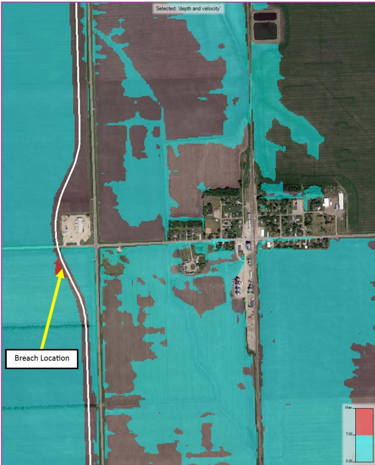
**Figure 17. Proposed Conditions Near-Vicinity Maximum D\*V for 90,000 cfs Event after Dam Breach at Location 3**
