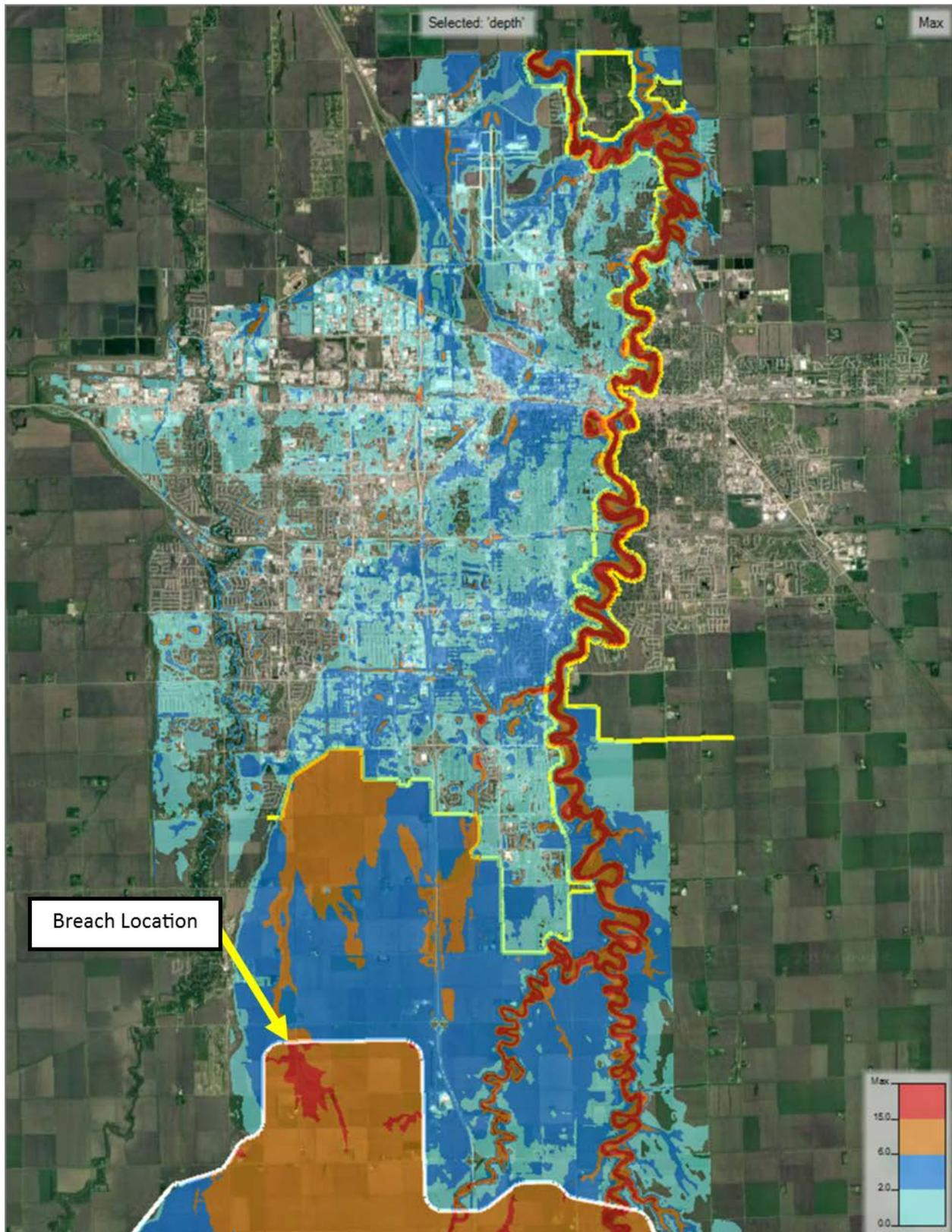
**Figure 9. Proposed Conditions Maximum Flow Depths for 90,000 cfs Event after Dam Breach at Location 1**
