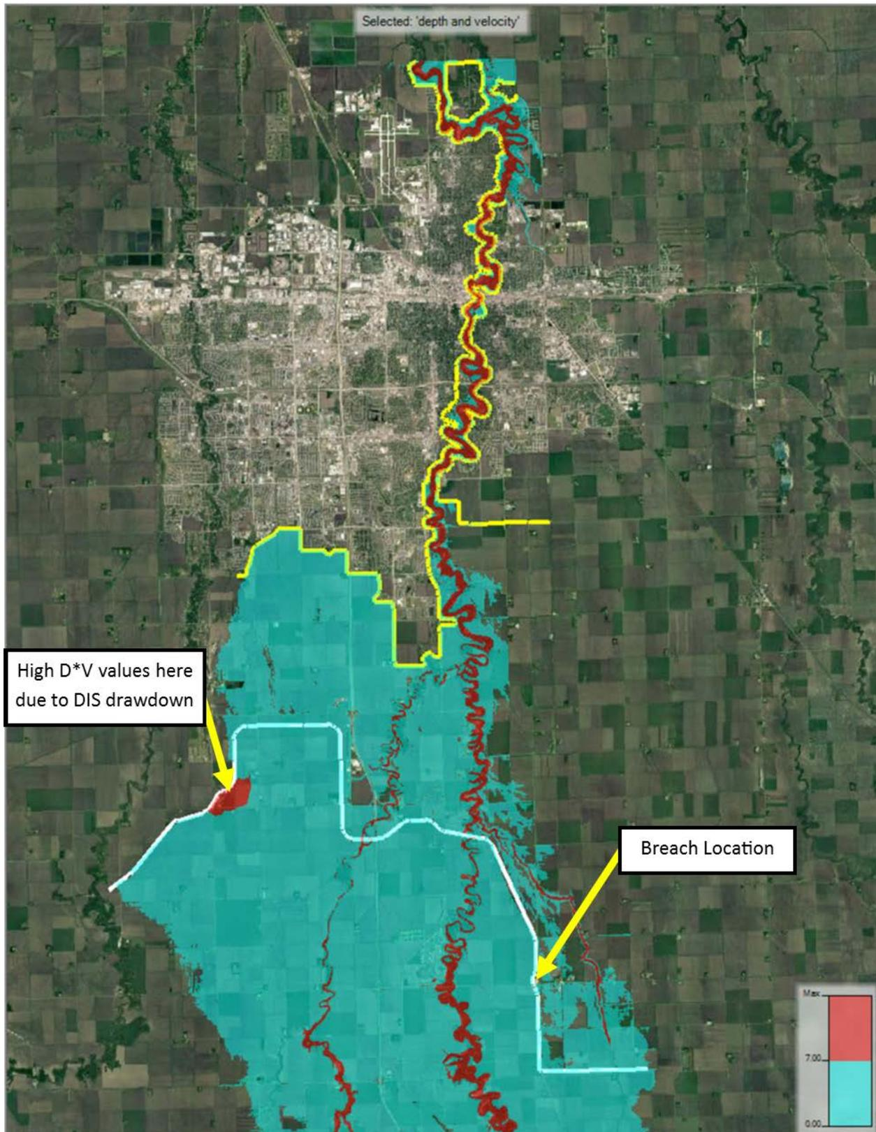
**Figure 16. Proposed Conditions Maximum D\*V for 90,000 cfs Event after Dam Breach at Location 3**
