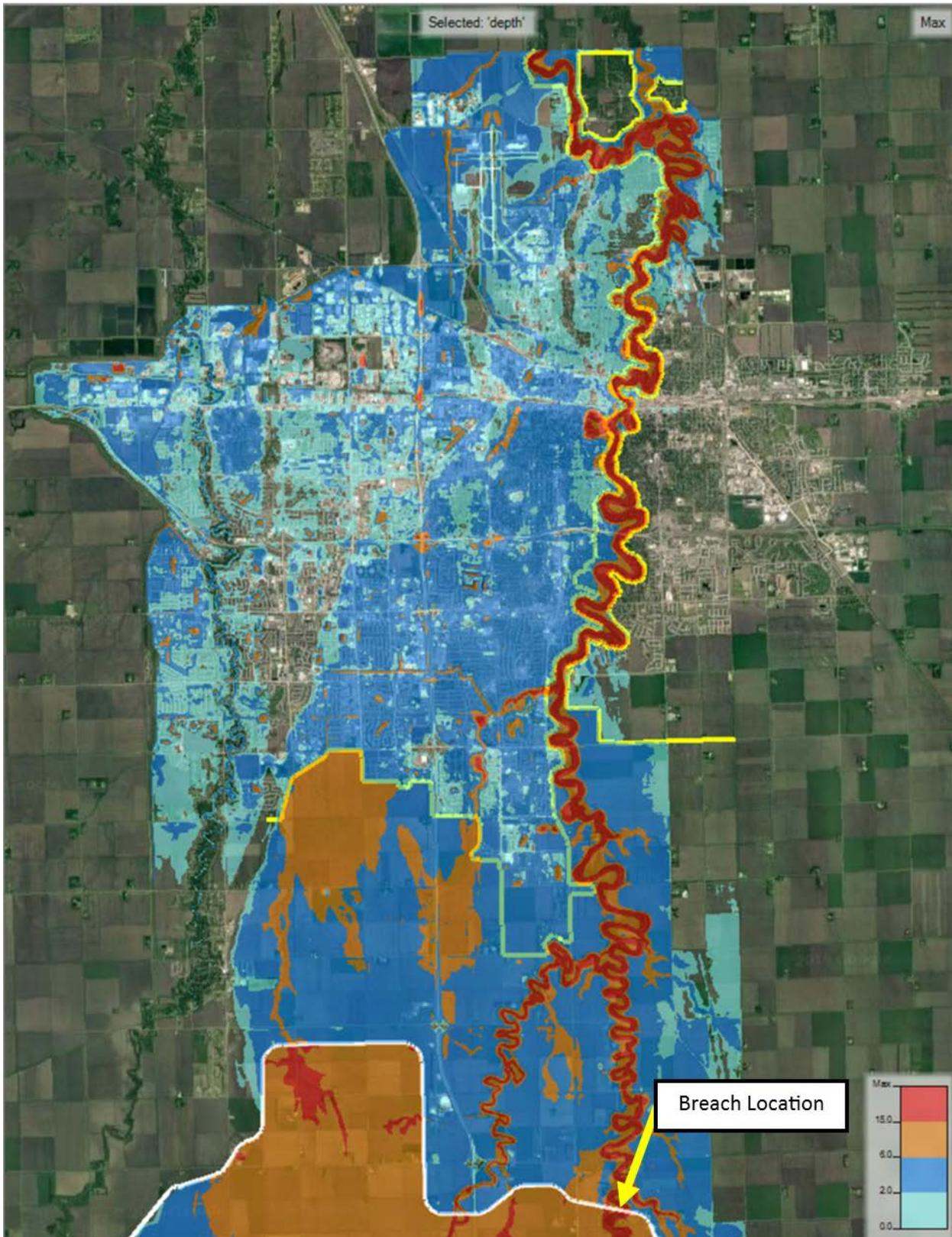
**Figure 21. Proposed Conditions Maximum Flow Depths for 90,000 cfs Event after Dam Breach at RRS**
