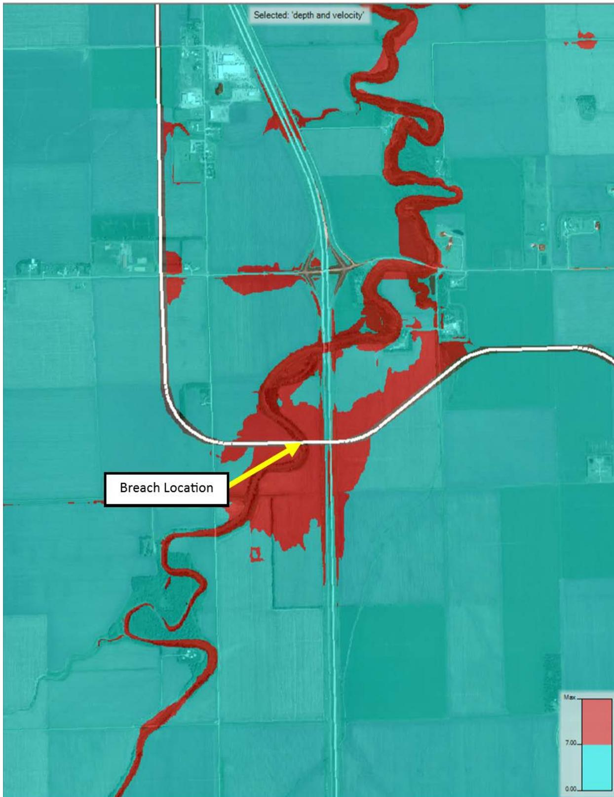
**Figure 20. Proposed Conditions Near-Vicinity Maximum  $D*V$  for 90,000 cfs Event after Dam Breach at WRRS**
