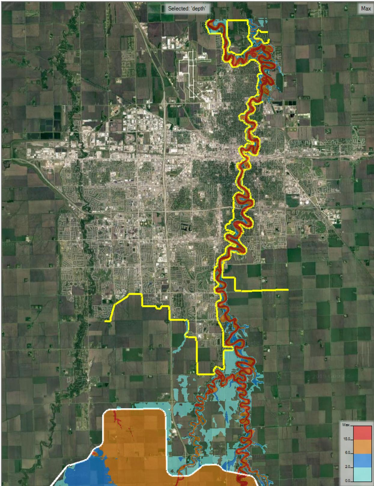
**Figure 29. Proposed Conditions Maximum Flow Depths for 1% ACE Event (No Dam or Levee Breach)**
