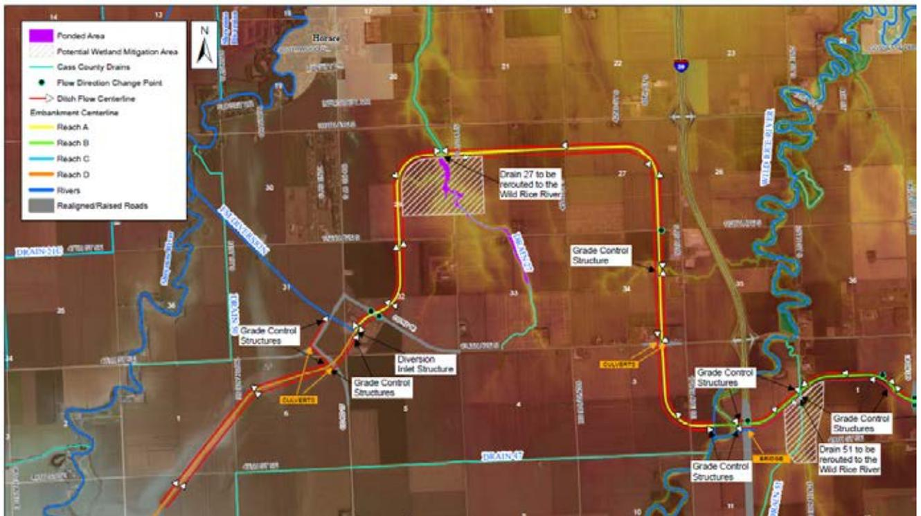
On the Minnesota side, the Dam/Southern Embankment has been realigned such that it follows relatively high ground from the Red River to Highway 75. Then, it extends south to a location
