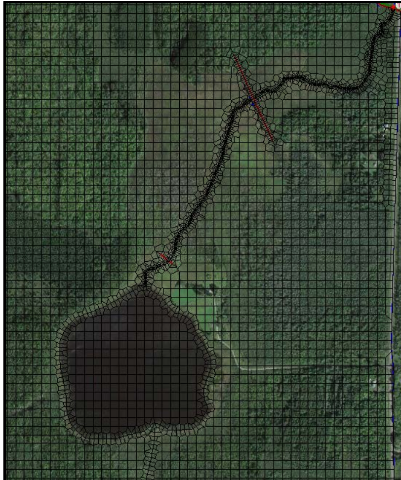
Figure 16: Flow area connections were used to represent beaver dams in the channel downstream of Cedar Lake.
