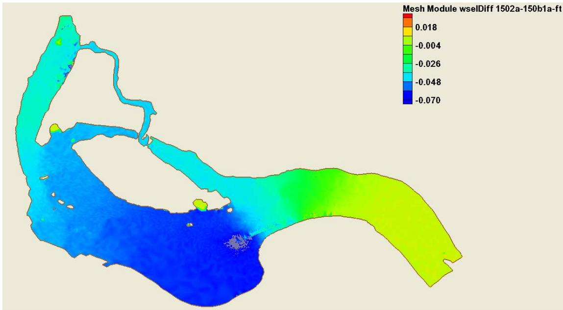
Figure C-4 Water Surface Elevation Change Above Base Conditions (100 Year) - 150000 cfs- Alternative 2a
