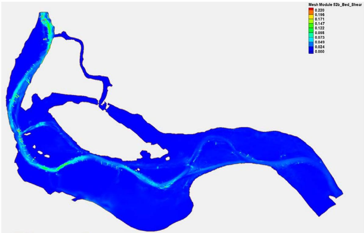
Figure C-5 Bed Shear (Low – 75% Duration) - 5970cfs - Alternative 2b
