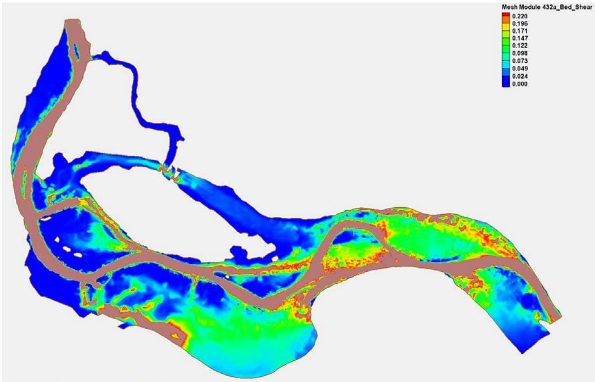
Figure C-14 Bed Shear (High - 2 Year) – 43000 cfs- Alternative 2a
