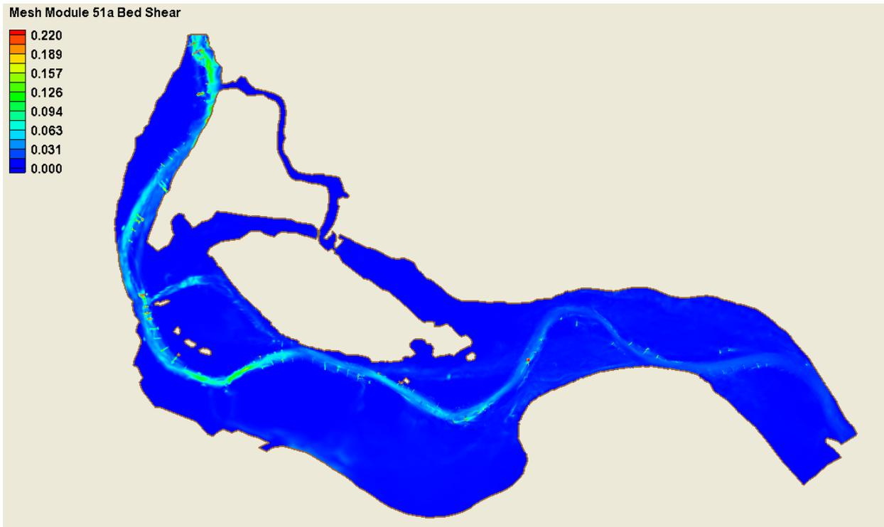
Figure C-2 Bed Shear (Low – 75% Duration) - 5970cfs - Alternative 1a
