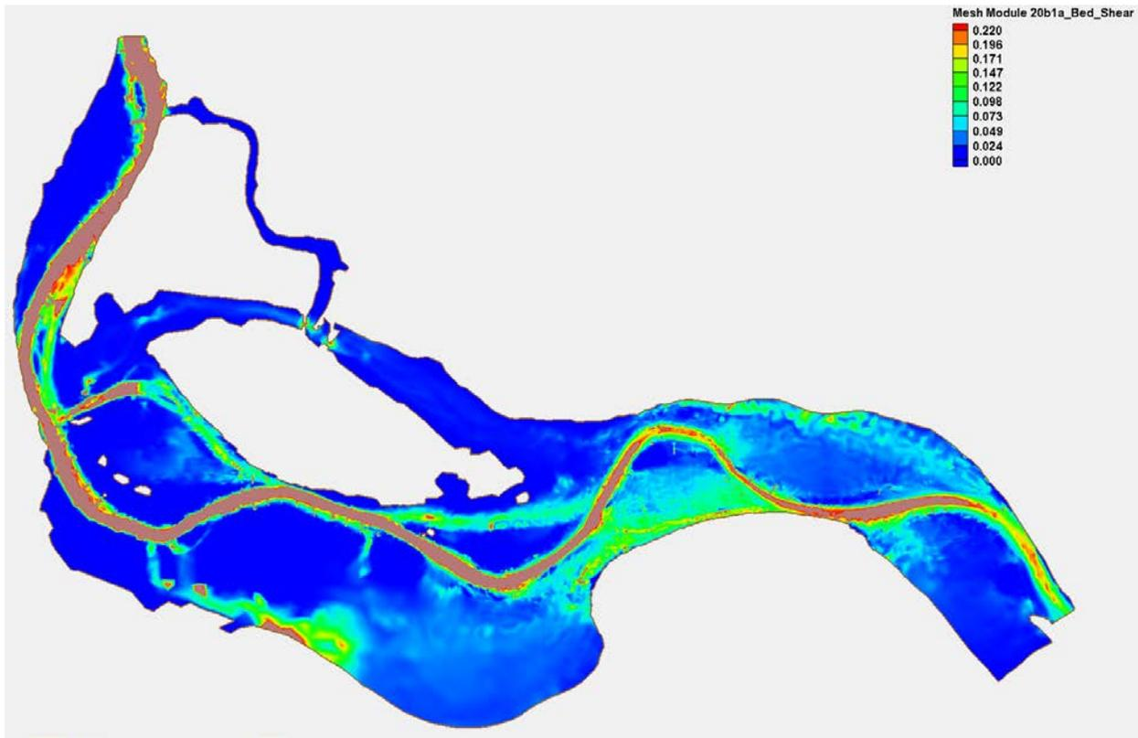
Figure C-6 Bed Shear (Medium - 25% Duration)- 20560 cfs- Base
