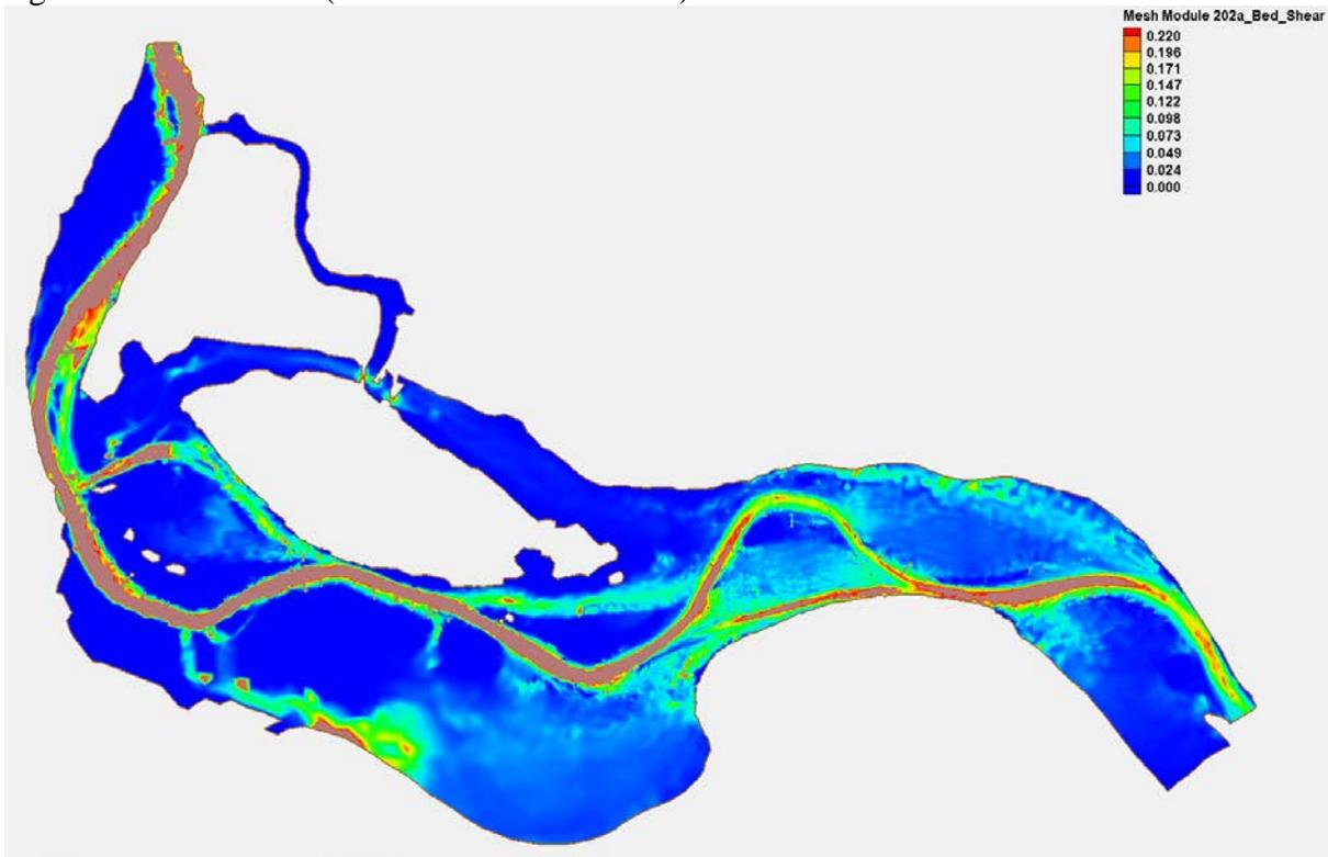
Figure C-9 Bed Shear (Medium - 25% Duration)- 20560 cfs- Alternative 2a
