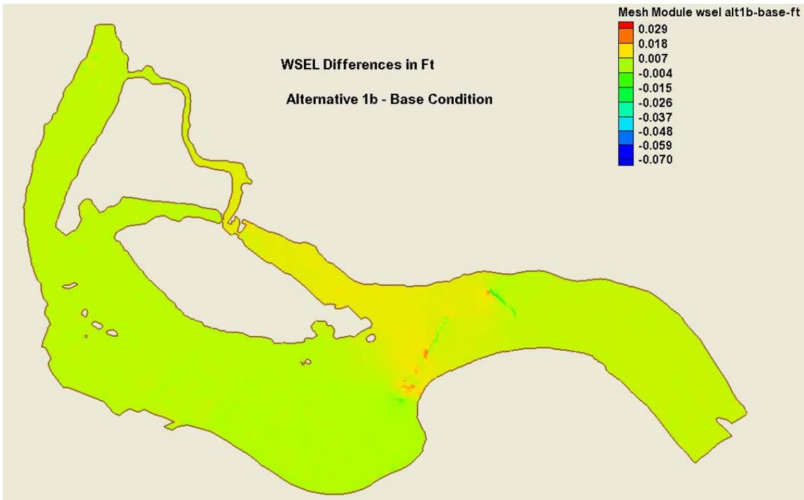
Figure C-3 Water Surface Elevation Change Above Base Conditions (100 Year) - 150000 cfs- Alternative 1b
