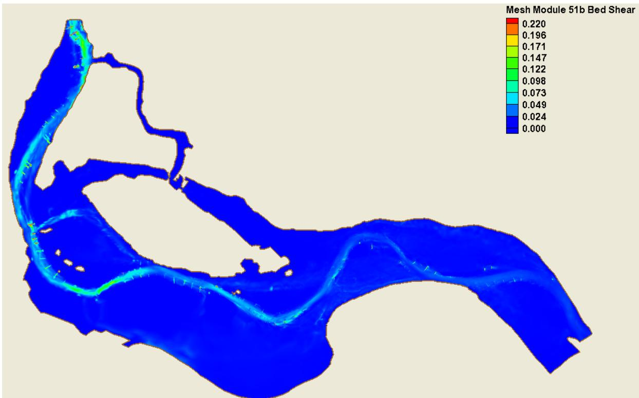
Figure C-3 Bed Shear (Low – 75% Duration) - 5970cfs - Alternative 1b
