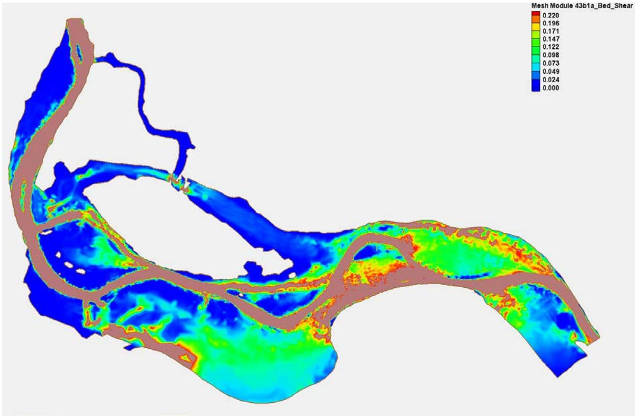
Figure C-11 Bed Shear (High - 2 Year) - 43000 cfs- Base
