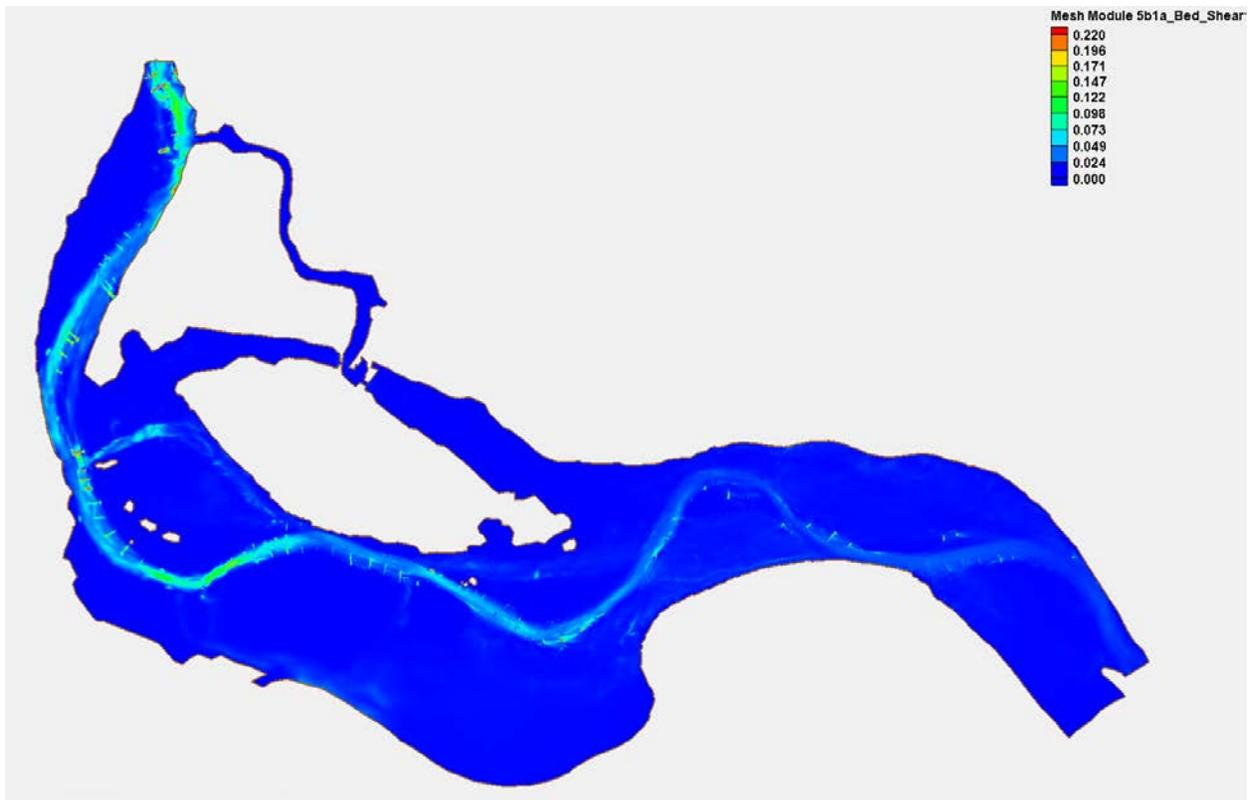
Figure C-1 Bed Shear (Low – 75% Duration) - 5970cfs – Base
