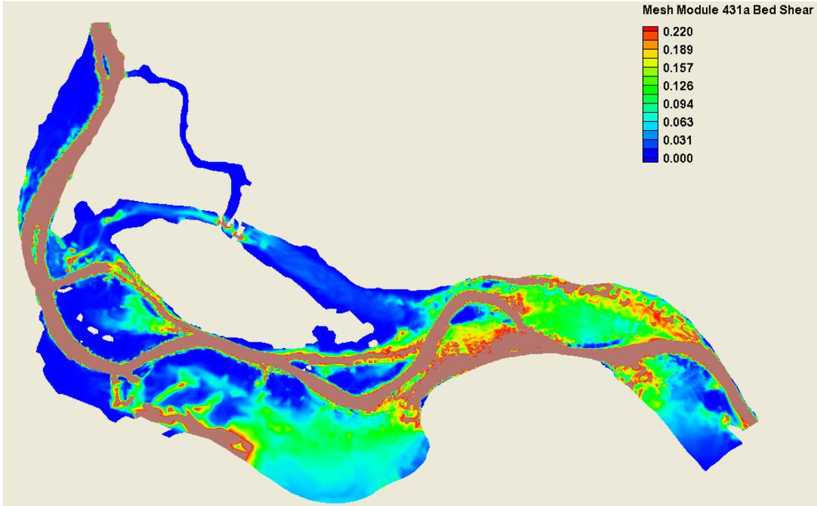
Figure C-12 Bed Shear (High - 2 Year) – 43000 cfs- Alternative 1a
