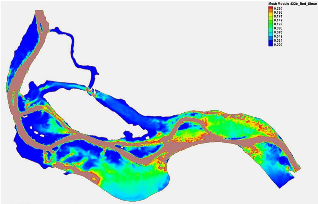
Figure C-15 Bed Shear (High - 2 Year) - 43000cfs- Alternative 2b
