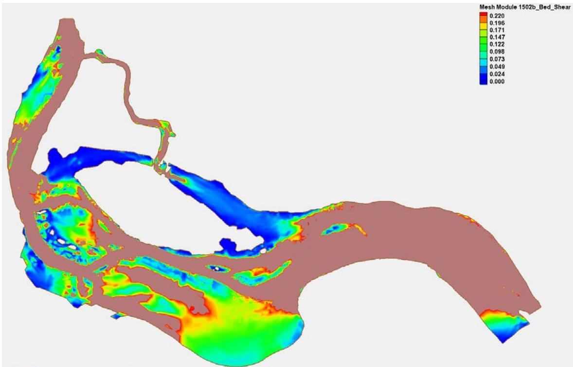
Figure C-20 Bed Shear (100 Year) - 150000 cfscfs- Alternative 2b
