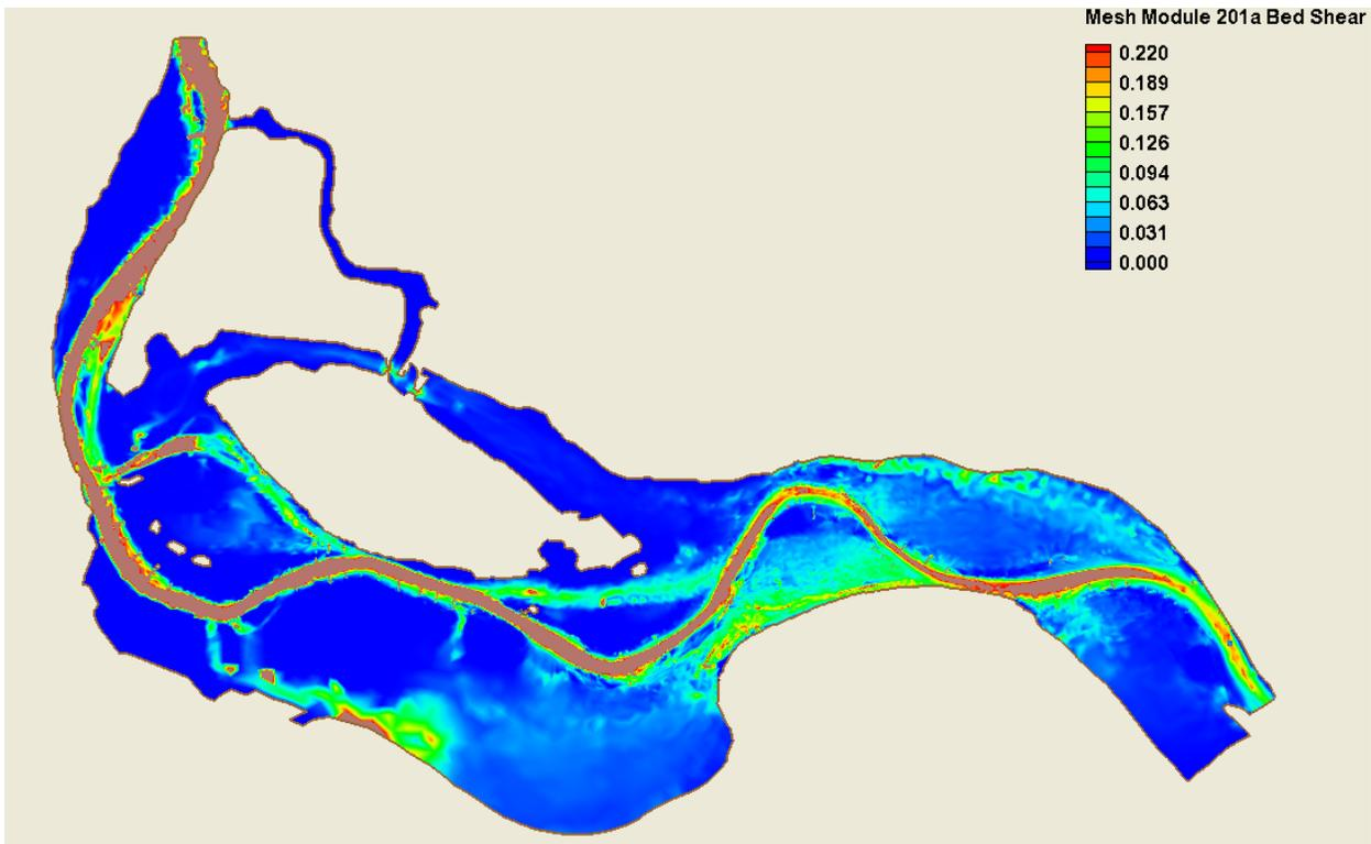
Figure C-7 Bed Shear (Medium - 25% Duration)- 20560 cfs- Alternative 1a
