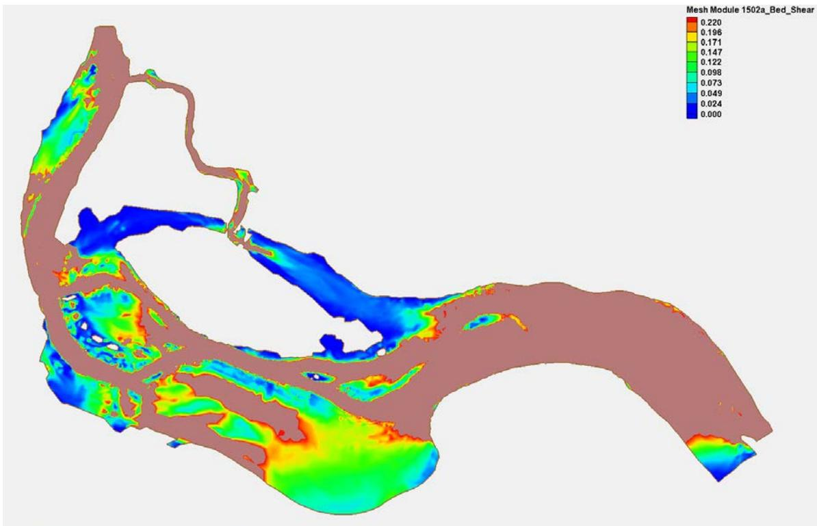
Figure C-19 Bed Shear (100 Year) - 150000 cfscfs- Alternative 2a
