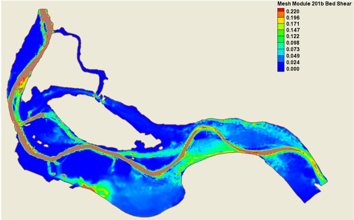
Figure C-8 Bed Shear (Medium - 25% Duration)- 20560 cfs- Alternative 1b
