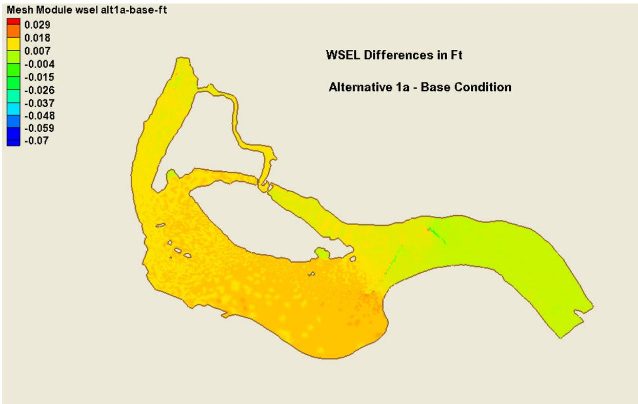
Figure C-2 Water Surface Elevation Change Above Base Conditions (100 Year) - 150000 cfs - Alternative 1a
