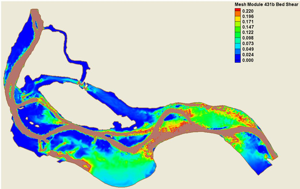
Figure C-13 Bed Shear (High - 2 Year) – 43000 cfs- Alternative 1b
