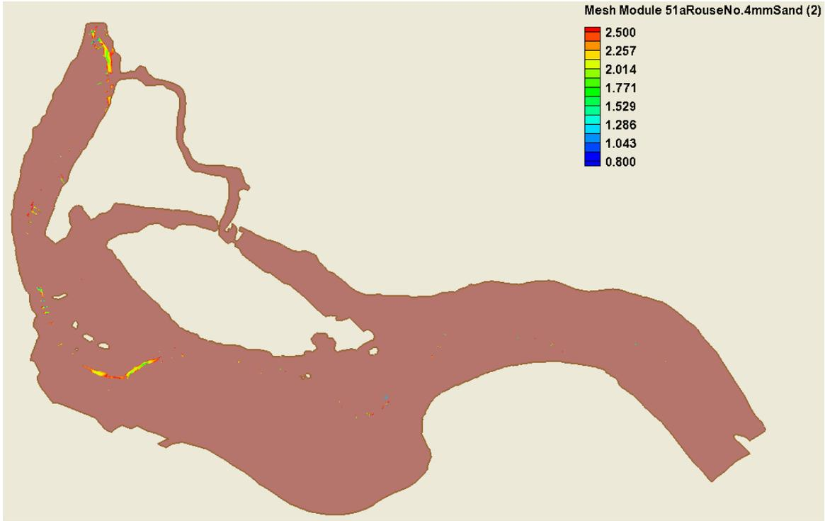
Figure C-22 Rouse (Low – 75% Duration) - 5970cfs - Alternative 1a
