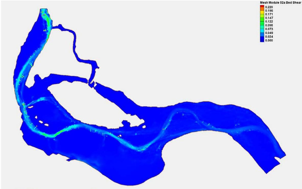
Figure C-4 Bed Shear (Low – 75% Duration) - 5970cfs - Alternative 2a
