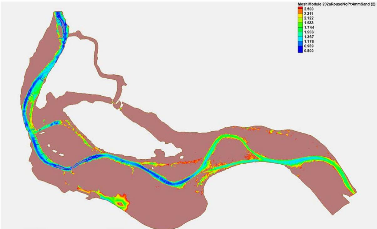
Figure C-4 Rouse (Medium - 25% Duration)- 20560 cfs- Alternative 2a
