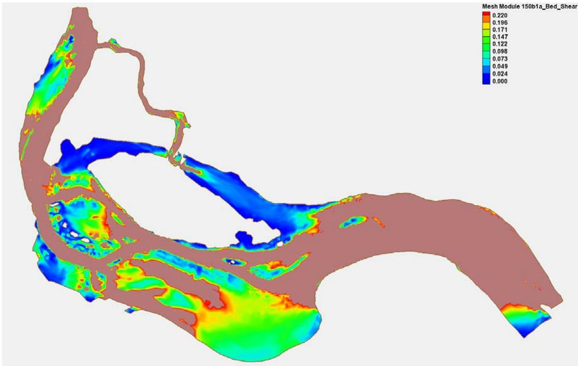
Figure C-16 Bed Shear (100 Year) - 150000 cfs cfs- Base
