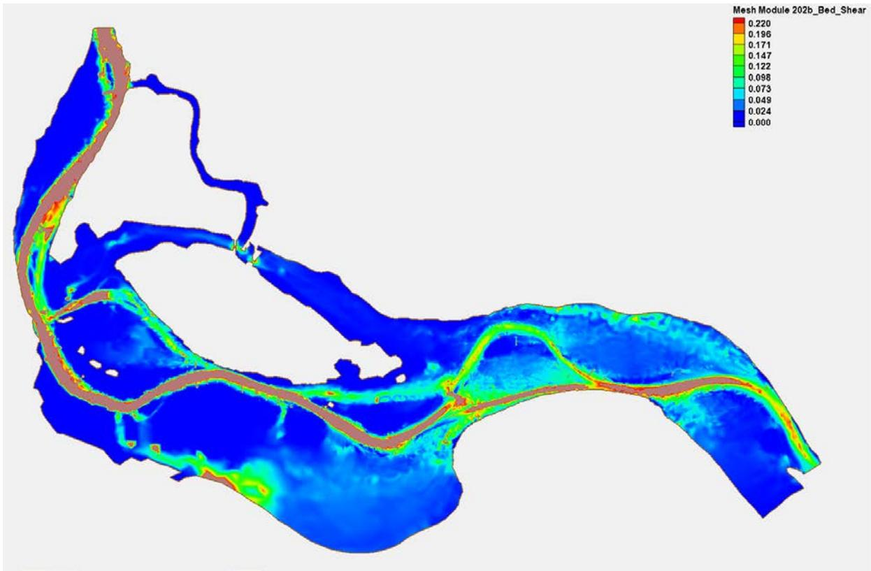
Figure C-10 Bed Shear (Medium - 25% Duration)- 20560 cfs- Alternative 2b
