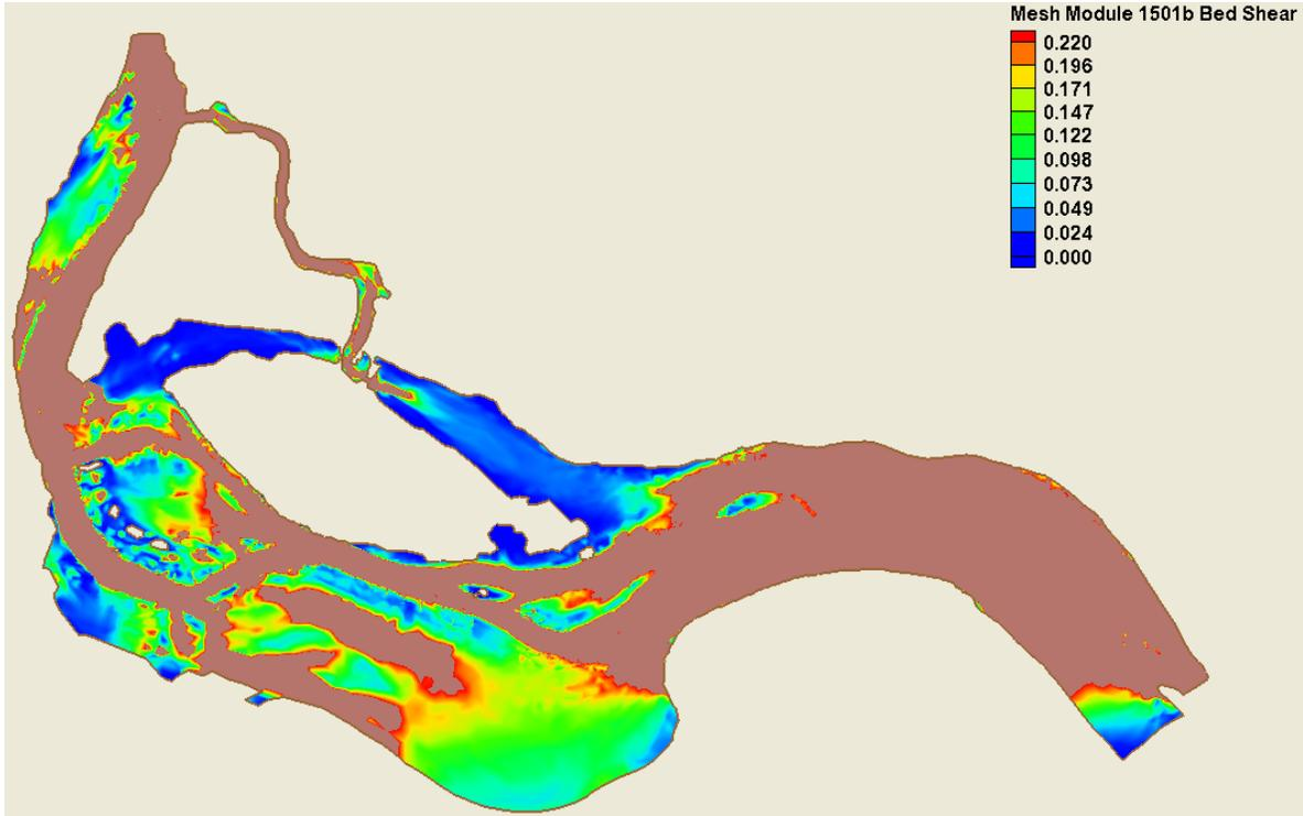
Figure C-18 Bed Shear (100 Year) - 150000 cfscfs- Alternative 1b
