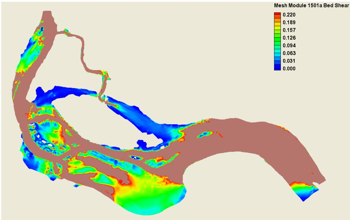
Figure C-17 Bed Shear (100 Year) - 150000 cfs cfs- Alternative 1a
