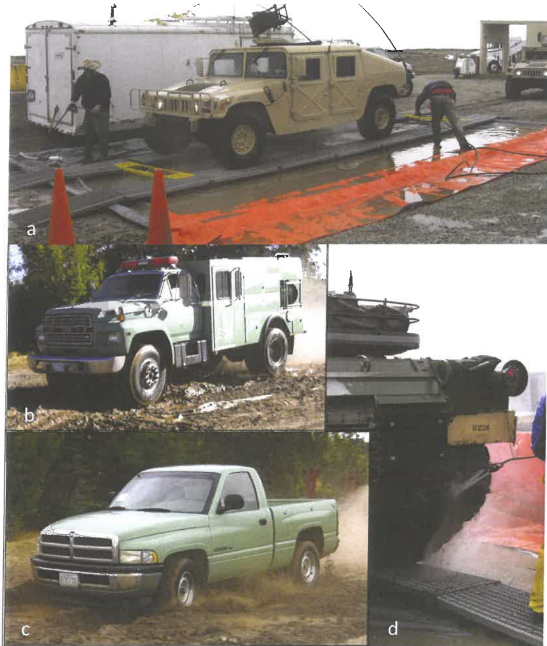
Fig. 1. The primary vehicle wash unit's (VWU) containment mats including raised edges, wheel racks, undercarriage washes and hand held wands are shown in a and d, and the artificially created mud bog used to evaluate VWU effectiveness is shown b and c. Vehicle types are as follows: 4WD (Humvee in a and truck in c), large 4WD in b, tracked - M1A1 tank in d.
