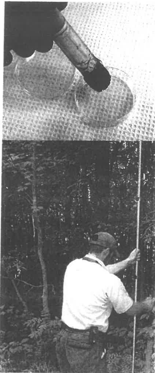
Fig. 2 Preparation and set up of passive samplers
