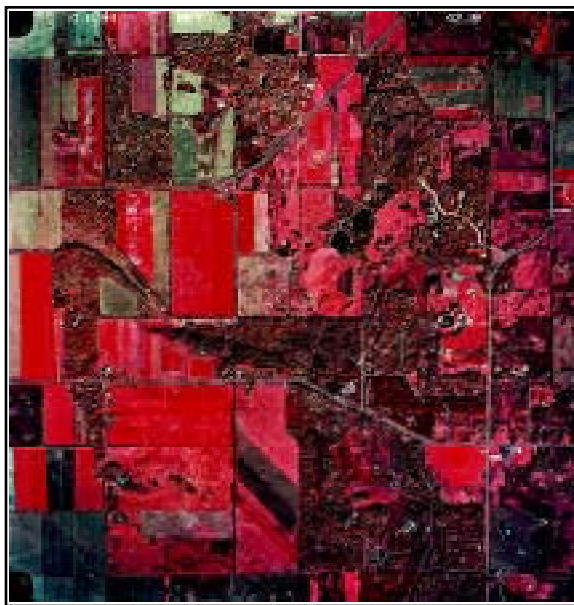
Figure 8. Infrared aerial photography is used by natural resource professionals to see patterns of water bodies, vegetation cover, and existing infrastructure.
