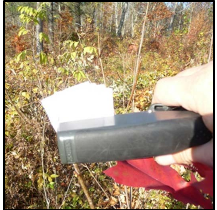
Step 6b: Staple once close to the stem nearly vertical, then a second time, forming an X or a crossed V.
