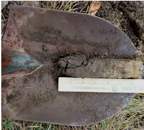
Photo 5. Trimming is complete, put the sample in a bucket.
