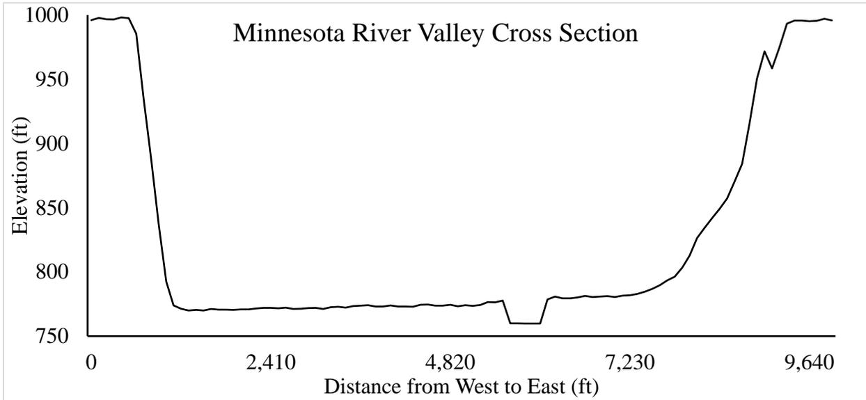
Mankato 1. Cross section elevation of the Minnesota River Valley near Mankato, MN derived from LiDAR data.
