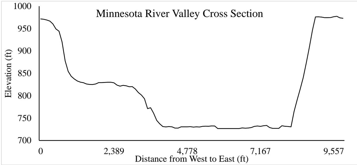
Henderson 1. Cross section elevation of the Minnesota River Valley near Henderson, MN derived from LiDAR data.
