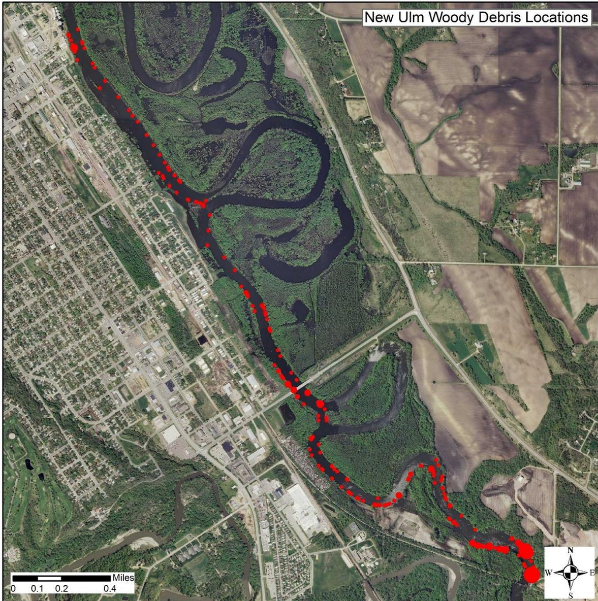
New Ulm 5. Map of the Minnesota River study site near New Ulm, MN showing locations of woody debris. The size of circles is proportional to the aerial coverage of woody debris.
