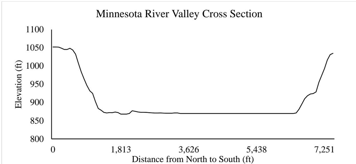
Upper Sioux 1. Cross section elevation of the Minnesota River Valley near Upper Sioux Agency State Park, Granite Falls, MN derived from LiDAR data.
