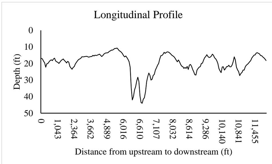
Shakopee 2. Longitudinal profile of the Minnesota River channel along the thalweg of a study site near Shakopee, MN.
