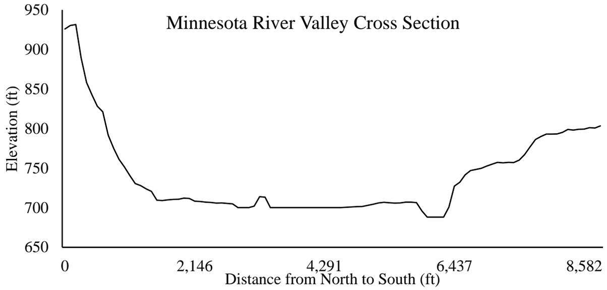
Shakopee 1. Cross section elevation of the Minnesota River Valley near Shakopee, MN derived from LiDAR data.
