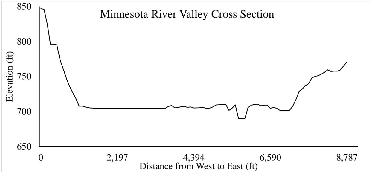
Chaska 1. Cross section elevation of the Minnesota River Valley near Chaska, MN derived from LiDAR data.
