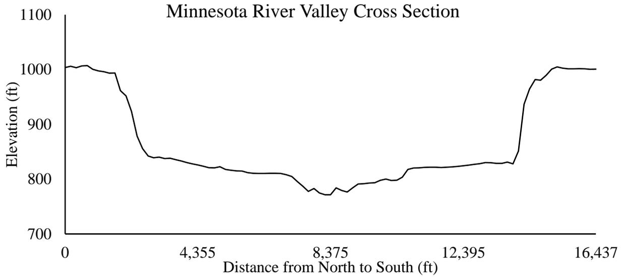
Judson 1. Cross section elevation of the Minnesota River Valley near Judson, MN derived from LiDAR data.
