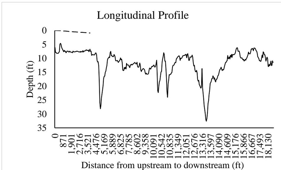
New Ulm 2. Longitudinal profile of the Minnesota River channel along the thalweg of a study site near New Ulm, MN.
