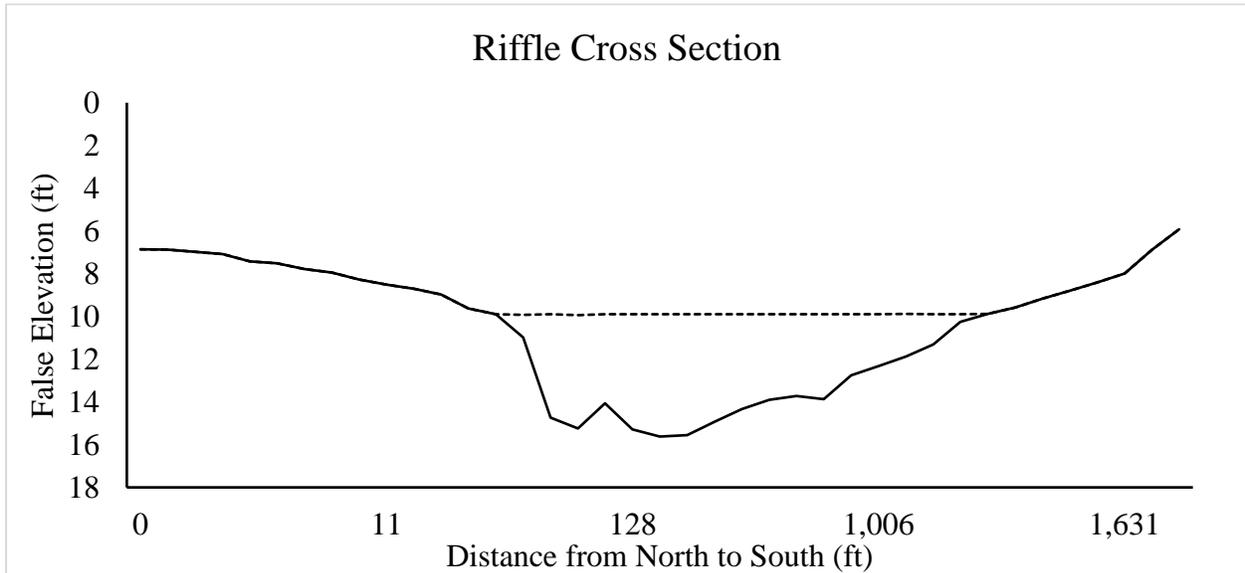
Montevideo 2. Surveyed cross section elevation of the Minnesota River at a riffle near Montevideo, MN.
