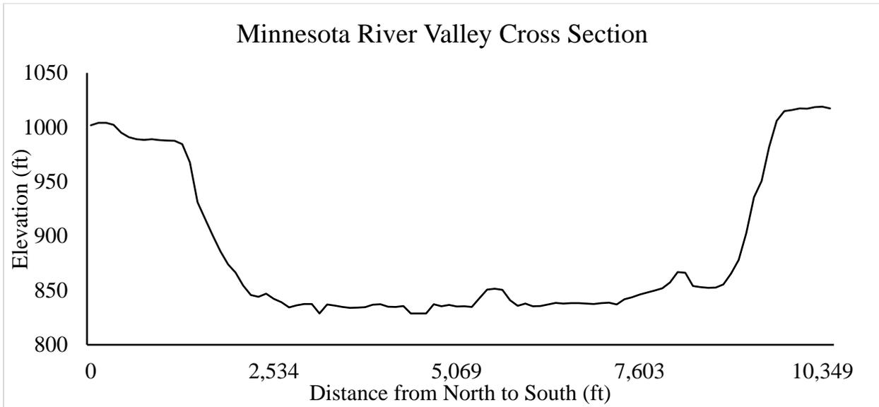
North Redwood 1. Cross section elevation of the Minnesota River Valley near North Redwood, MN derived from LiDAR data.
