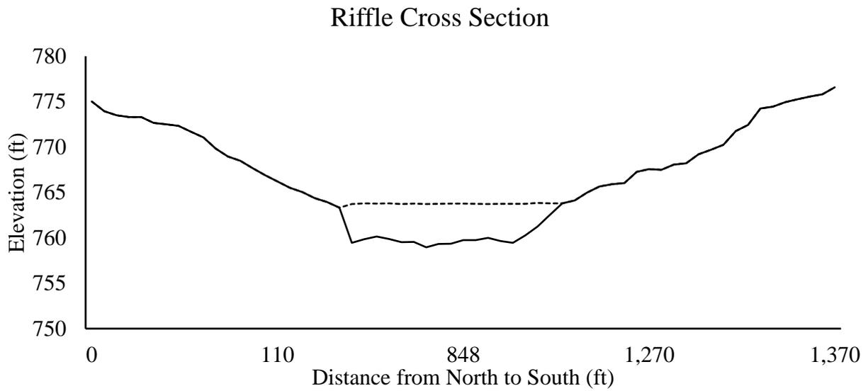
Judson 2. Surveyed cross section elevation of the Minnesota River at a riffle near Judson, MN.
