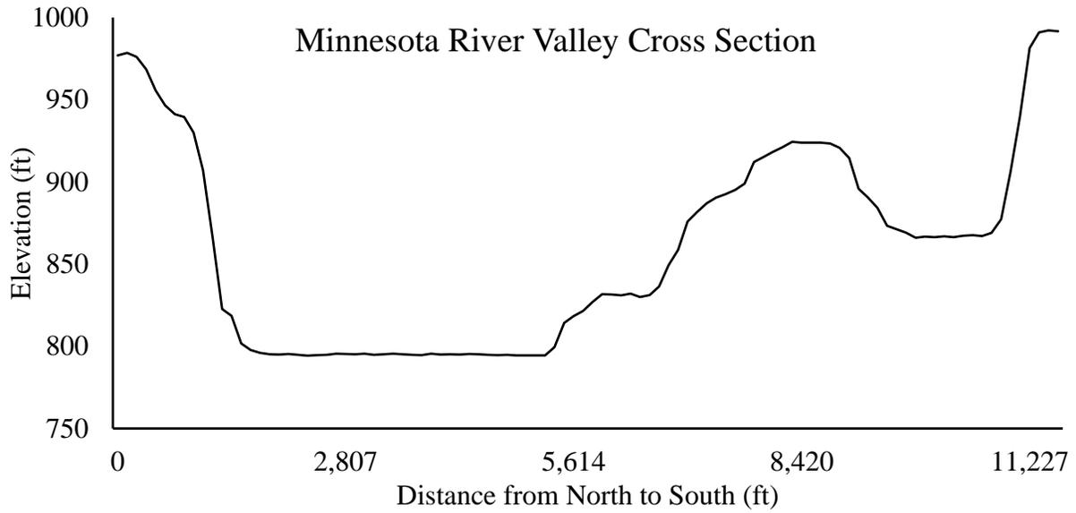
New Ulm 1. Cross section elevation of the Minnesota River Valley near New Ulm, MN derived from LiDAR data.
