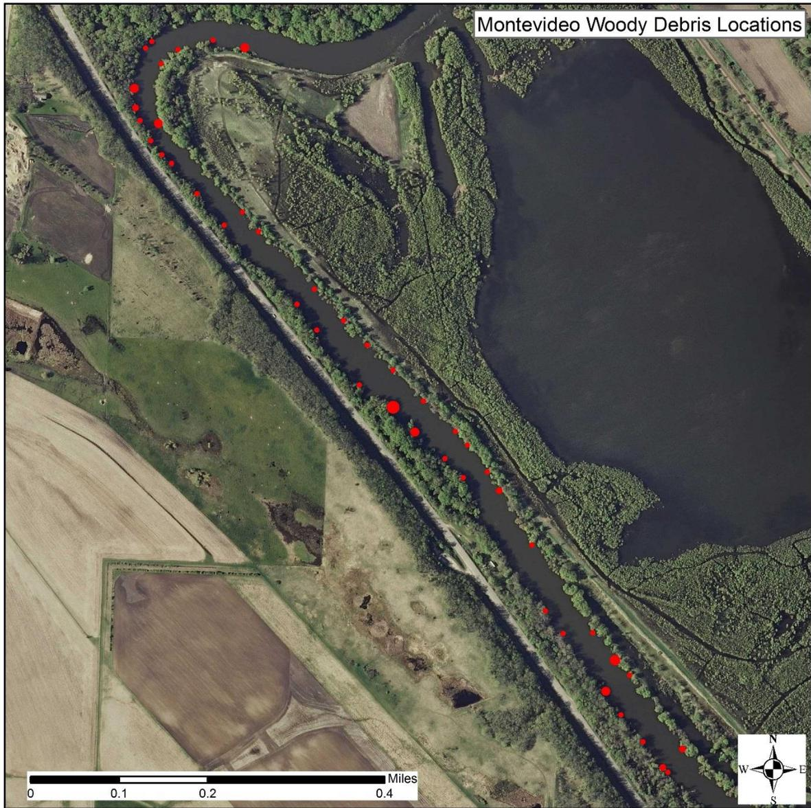
Montevideo 6. Map of the Minnesota River study site near Montevideo, MN showing locations of woody debris. The size of circles is proportional to the aerial coverage of woody debris.
