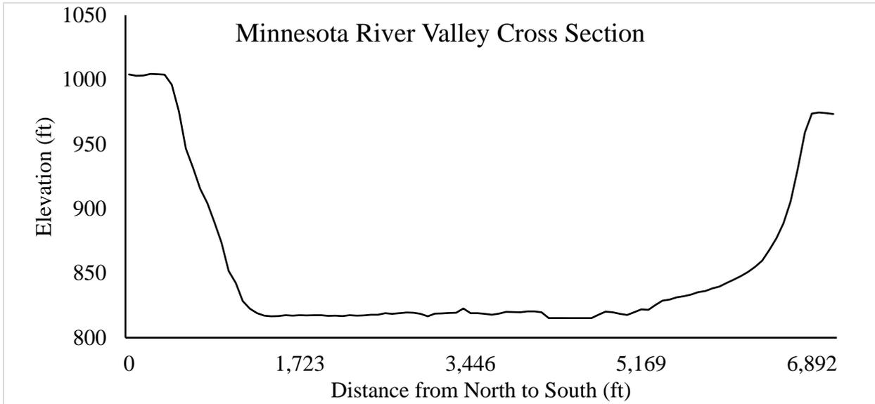
Franklin 1. Cross section elevation of the Minnesota River Valley near Franklin, MN derived from LiDAR data.
