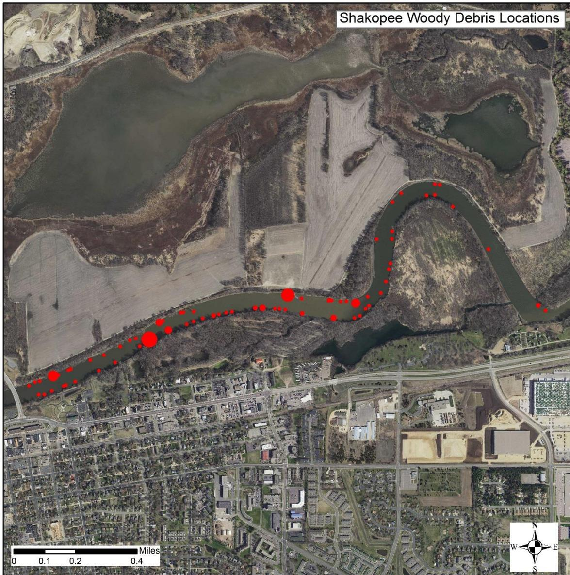
Shakopee 5. Map of the Minnesota River study site near Shakopee, MN showing locations of woody debris. The size of circles is proportional to the aerial coverage of woody debris.
