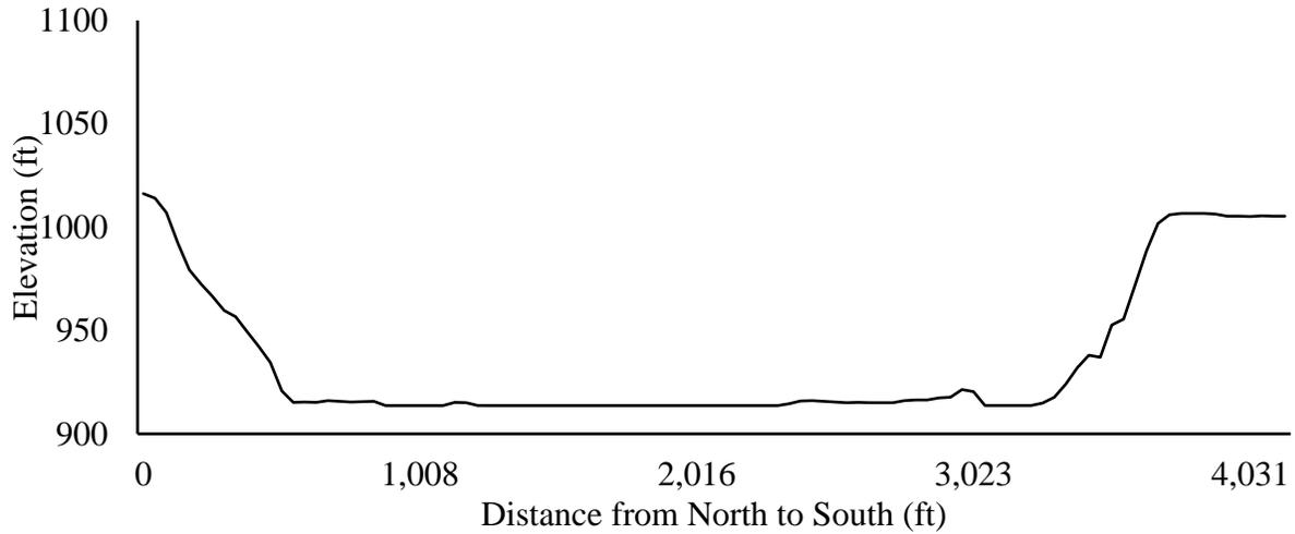
Montevideo 1. Cross section elevation of the Minnesota River Valley near Montevideo, MN derived from LiDAR data.
