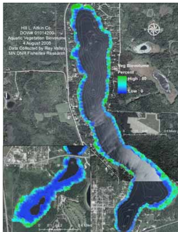
Figure 6. Aquatic vegetation biovolume (percent of water column occupied by vegetation) assessed on Hill Lake with hydroacoustics during August 2008
