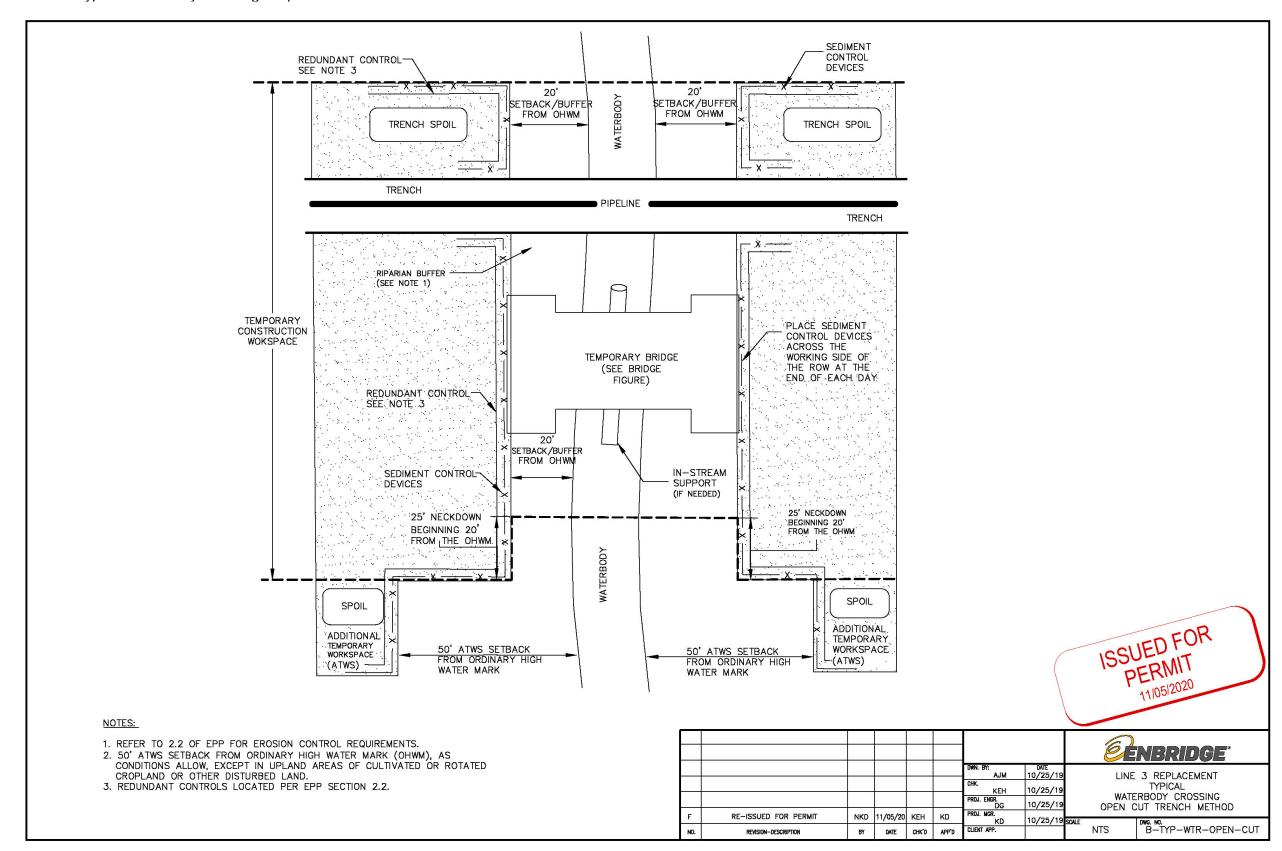
Figure 23 Typical Waterbody Crossing – Dam and Pump Method
