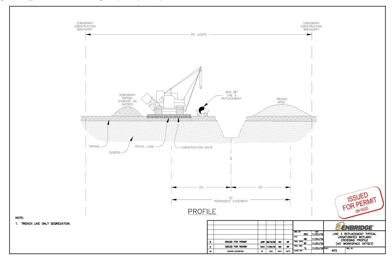
Figure 32 Typical Saturated Wetland Crossing Profile (25' workspace offset)
