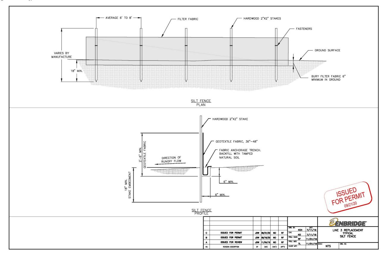
Figure 7 Typical Super Silt Fence
