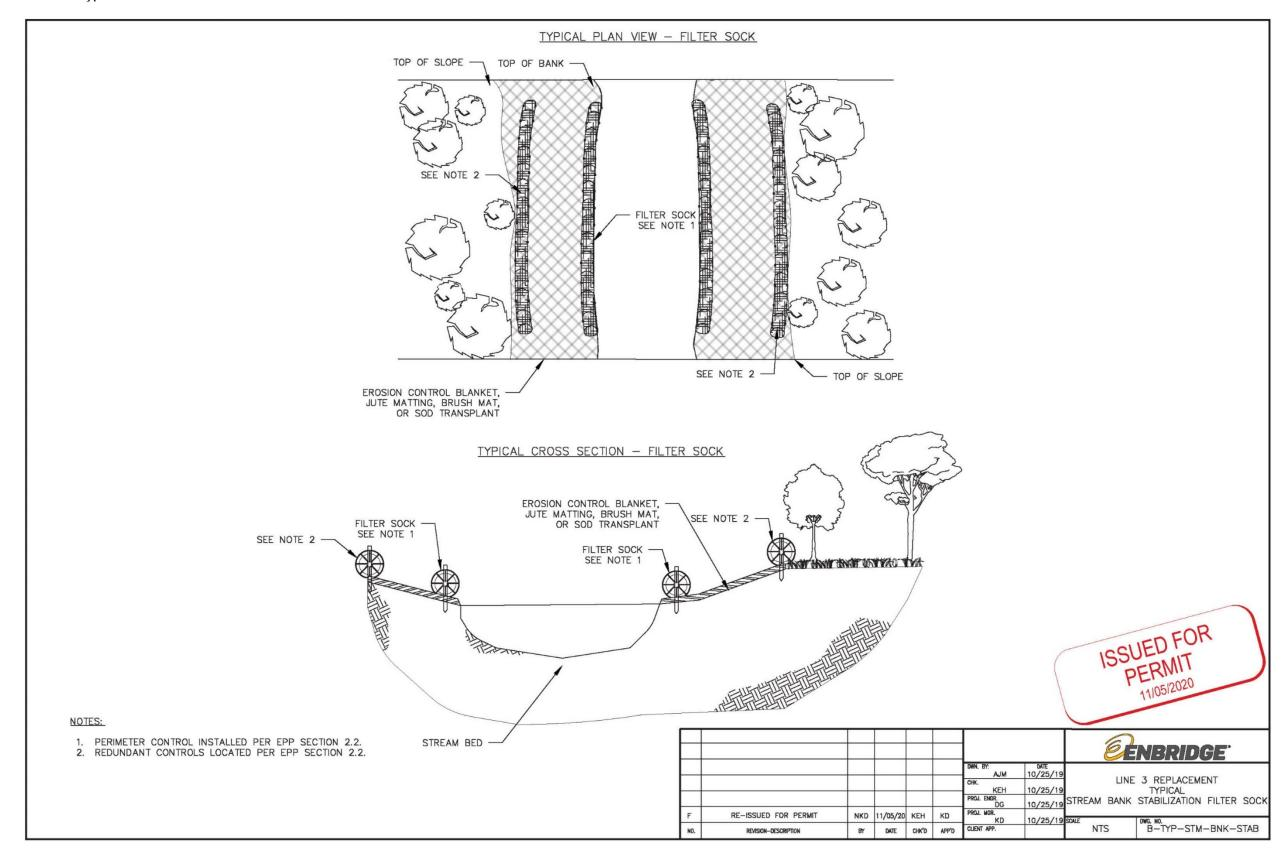
Figure 28 Typical Final Stream Bank Stabilization & Erosion Control
