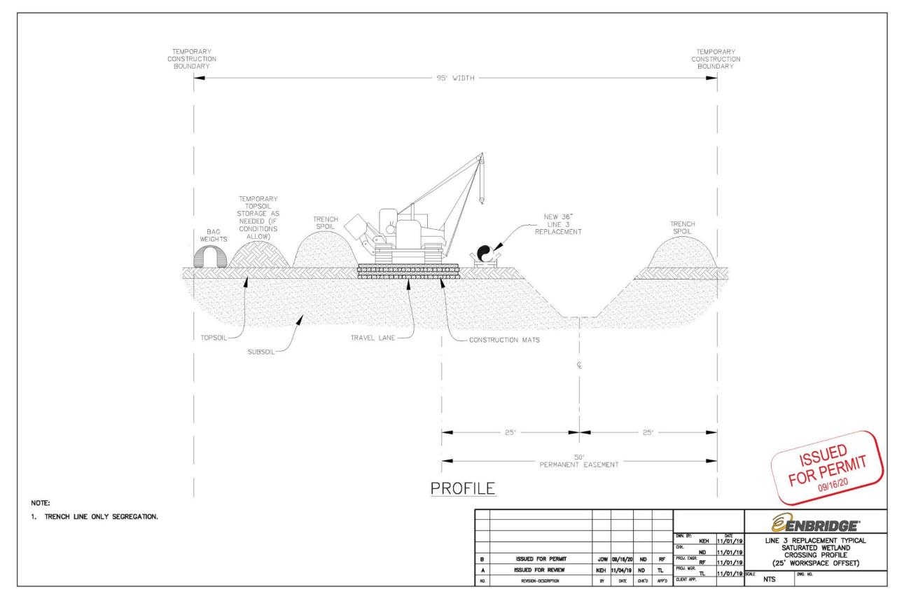
Figure 33 Typical Saturated Wetland Crossing Profile (40' workspace offset)
