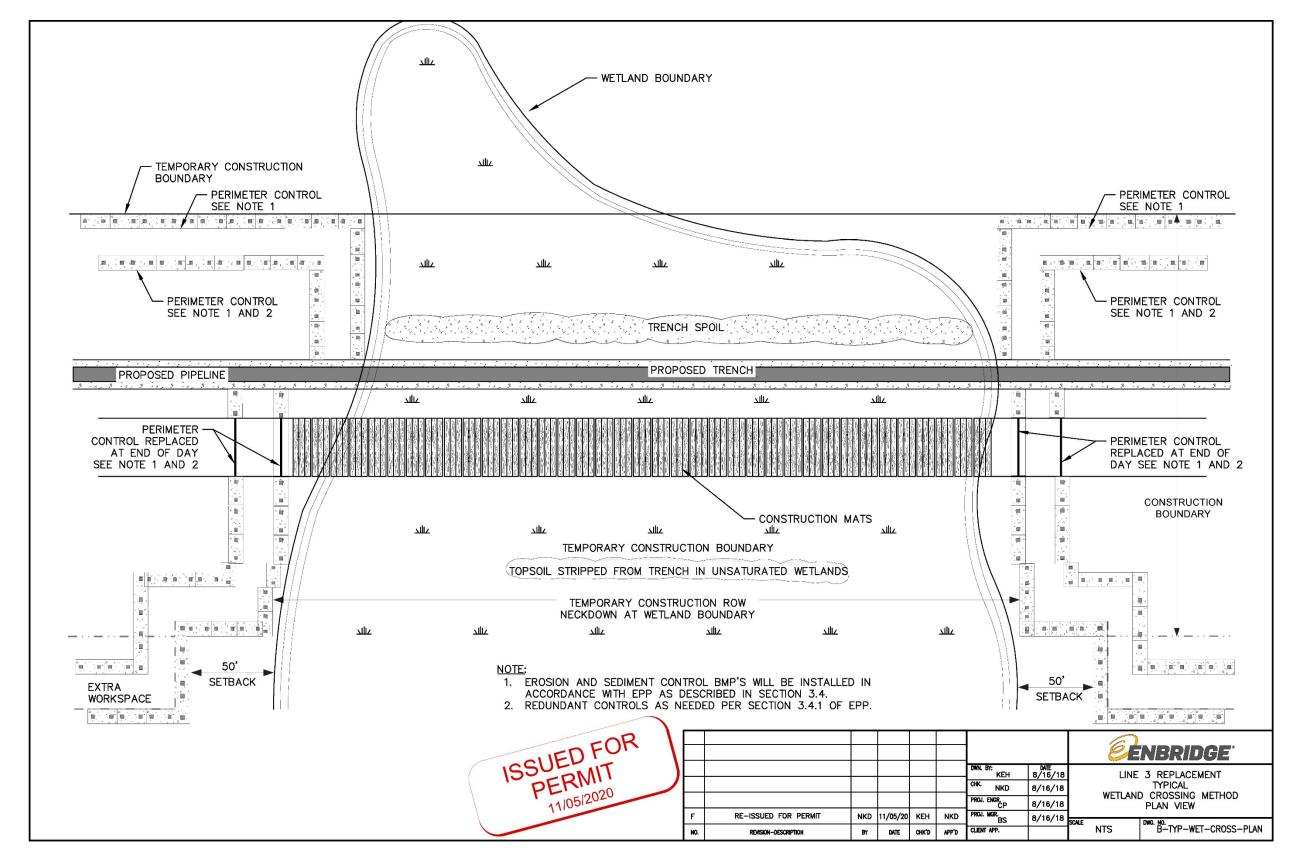
Figure 35 Typical Push-Pull Method – Saturated Wetland (25' workspace offset)
