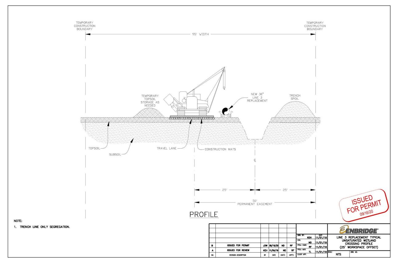
Figure 31 Typical Unsaturated Wetland Crossing Profile (40' workspace offset)
