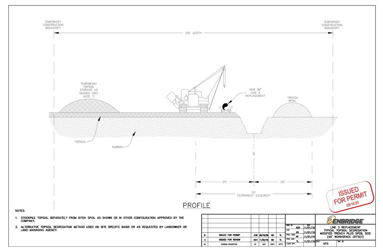
Figure 18 Typical Trench and Backfill Requirements
