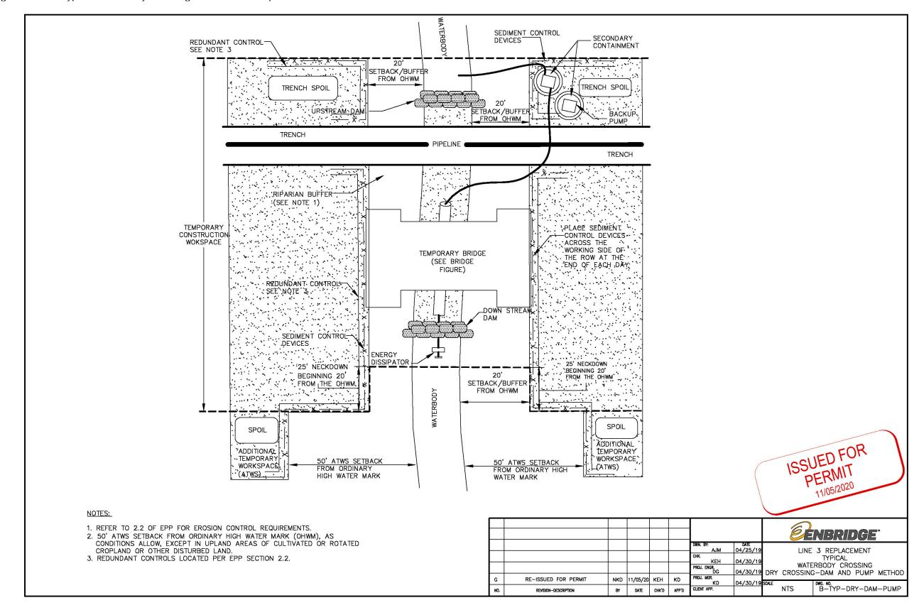
Figure 24 Typical Waterbody Crossing – Flume Method
