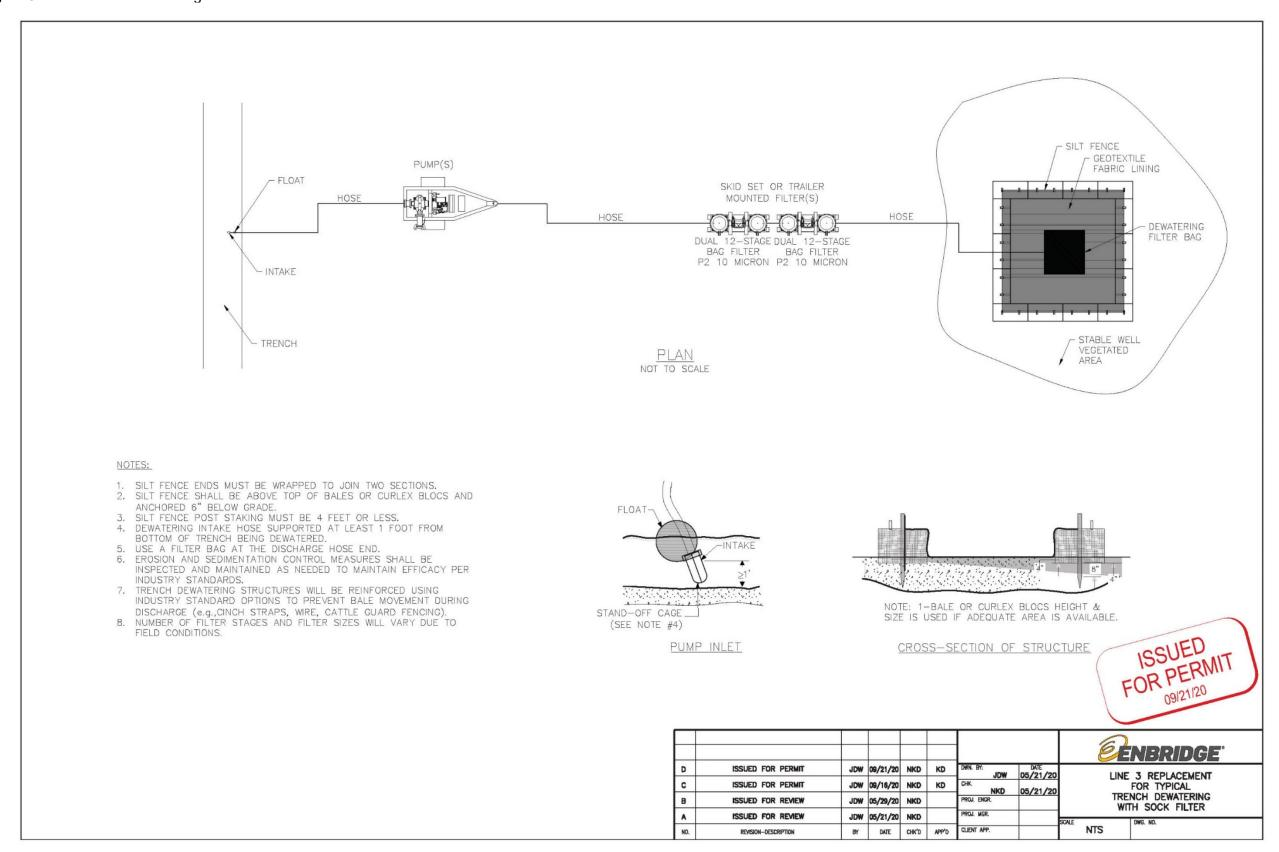
Figure 55 Trench Dewatering with Sand Filter
