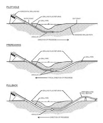
Figure 3.6-1: General Stages of an HDD
