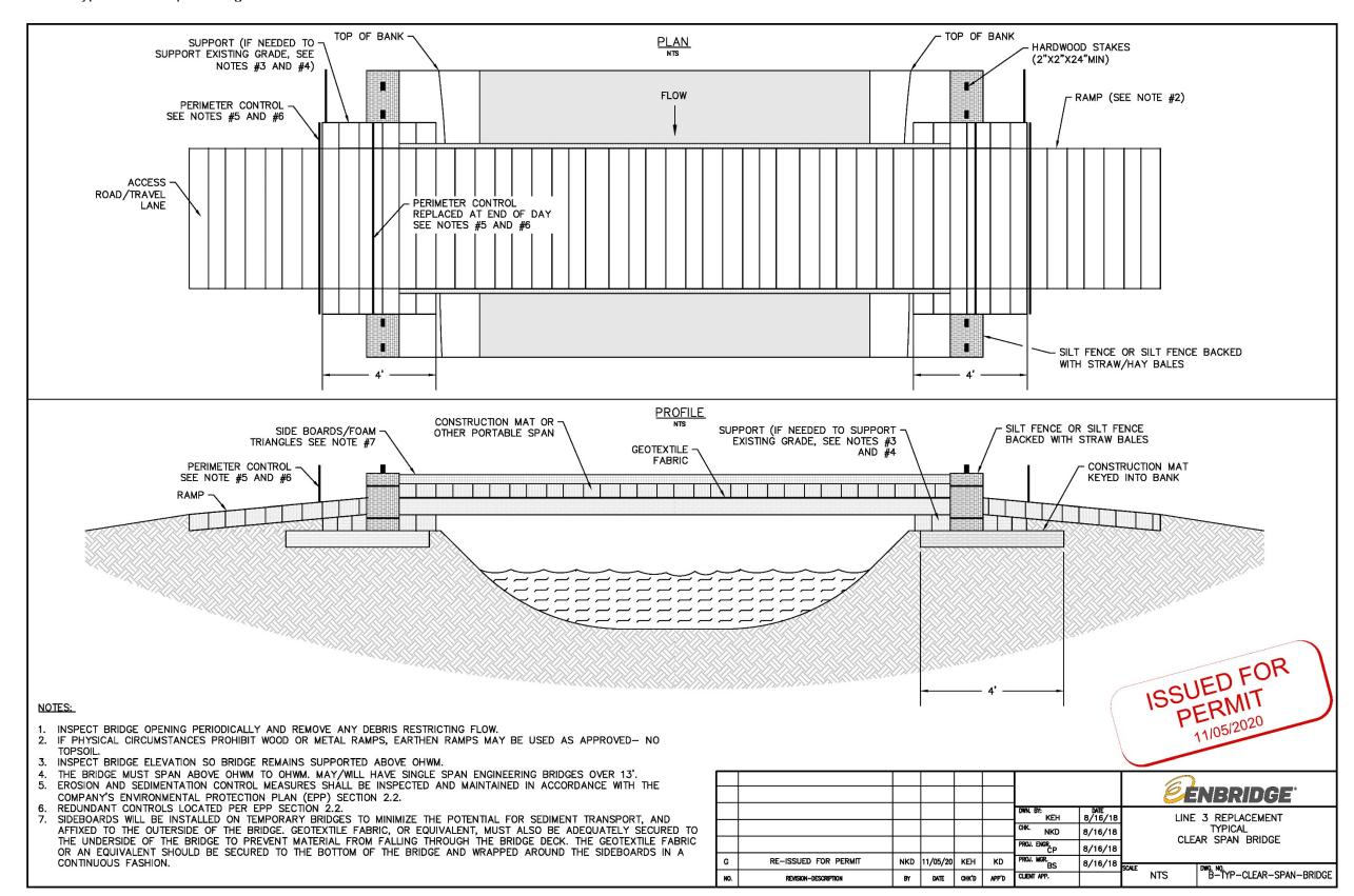
Figure 4 Typical Non-Clear Span Bridge
