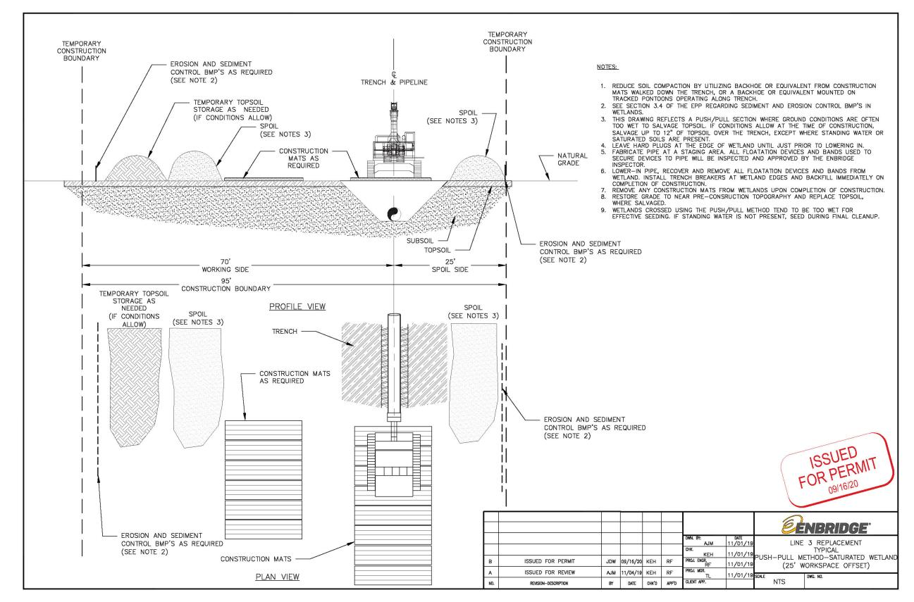
Figure 36 Typical Push-Pull Method – Saturated Wetland (40' workspace offset)
