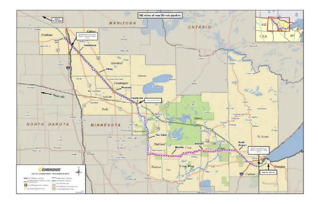
7. The Project proposes to maintain a 50-foot wide permanent corridor along the pipeline route. During construction, the Project proposes to temporarily widen the corridor to 120-feet wide in uplands and 95-feet wide in wetlands. The pipeline route also includes additional temporary construction workspaces ("ATWS").
