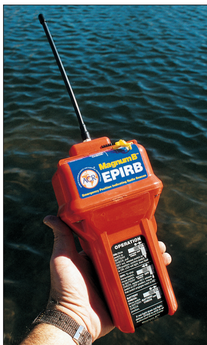
When activated, an EPIRB broadcasts an S.O.S. via satellite to rescue units on the ground.
