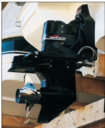
The inboard-outdrive (left) offers the power of an inboard engine and the flexibility of an outboard. An inboard boat (right) is steered by means of a rudder located behind the propeller.
