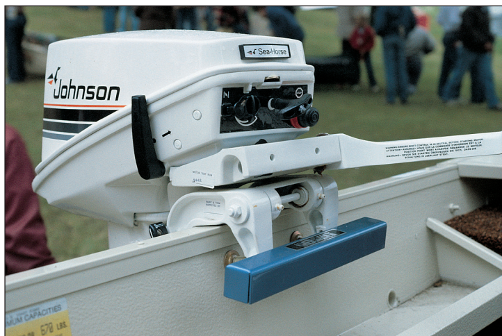
Outboard motors are popular targets of thieves. A bar lock such as this one makes theft much more difficult.
