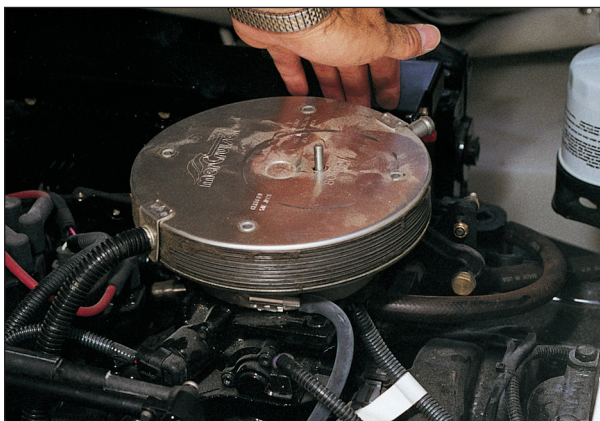
A flame arrester prevents backfires from entering the engine compartment.
