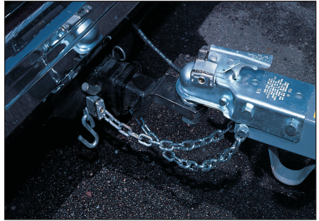
Hitches should be firmly attached to car frame. Safety chains are crossed so the coupling will not fall to the road if the trailer comes unhitched.
