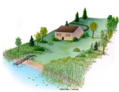
Buffer zones reduce runoff and erosion.
