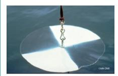
A Secchi disc measures the clarity of the water.
