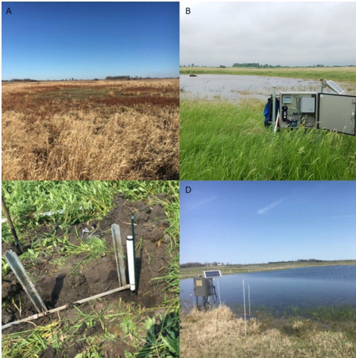
Figure A76: (A) View of Prairie WMA 1 on November 3, 2020. (B) View of the wetland on June 9, 2020, when bubbler equipment began collecting data. (C) PVC well housing bubbler transducer, taken on August 18, 2021. (D) View of the wet meadow on May 10, 2022, when OTT equipment was installed.
