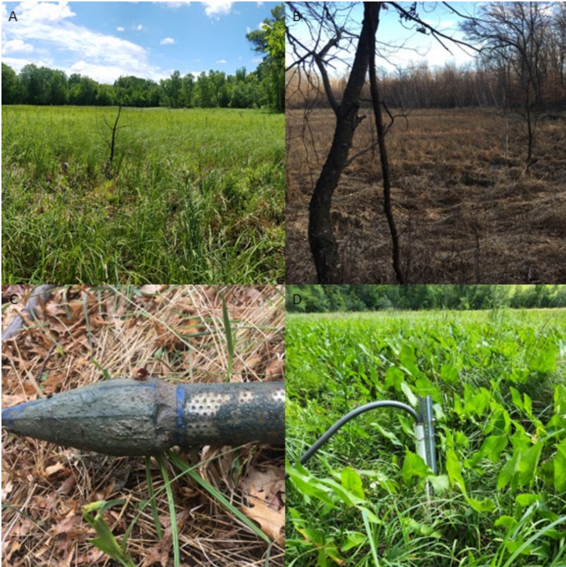
Figure A51: (A) View of Lake Maria State Park 3 on June 10, 2020. (B) Steel well housing bubbler transducer (right side of photo) in the wet meadow, taken on March 31, 2021. (C) Sand-point on the bottom of steel well, taken on May 26, 2022. (D) PVC well housing OTT transducer, taken on August 11, 2022.
