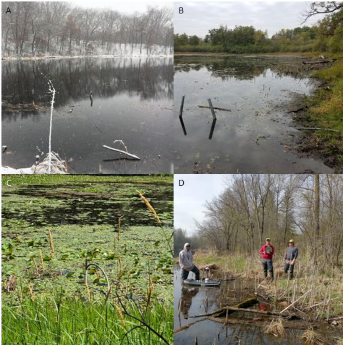
Figure A61: (A) View of Murphy Hanrehan Park Reserve 1 on November 12, 2020. (B) Fence posts supporting bubbler transducer, taken on October 6, 2021. (C) PVC pipe housing OTT transducer, taken on July 14, 2022. (D) Conducting a bathymetric survey on April 28, 2021.
