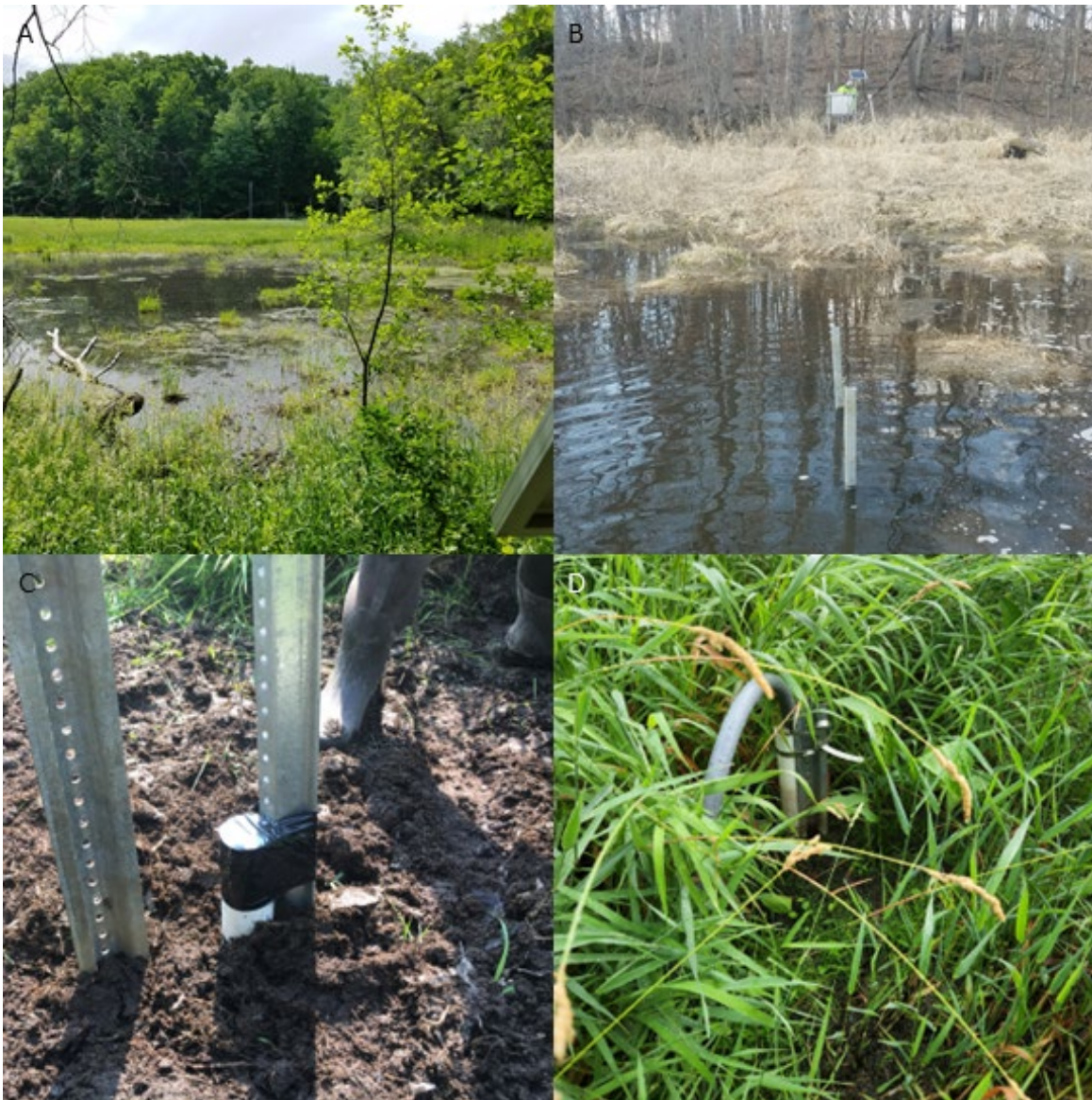
Figure A41: (A) View of Lake Maria State Park 1 on June 10, 2020. (B) Fence posts supporting first set of bubbler equipment, facing steel housing with loggers, taken on March 31, 2021. (C) New bubbler equipment in PVC well, installed adjacent to original equipment (fence post on left), taken on July 15, 2021. (D) PVC well housing OTT equipment, taken on July 13, 2022.
