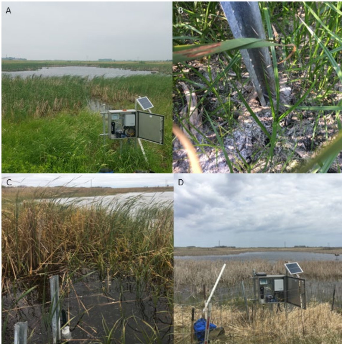
Figure A81: (A) View of Prairie WMA 2 on June 9, 2020. (B) Fence post supporting bubbler equipment and no water above ground on August 18, 2021. (C) Fence posts supporting bubbler equipment (including PVC well) with inundation on October 14, 2021. (D) Installation of OTT equipment on May 10, 2022.
