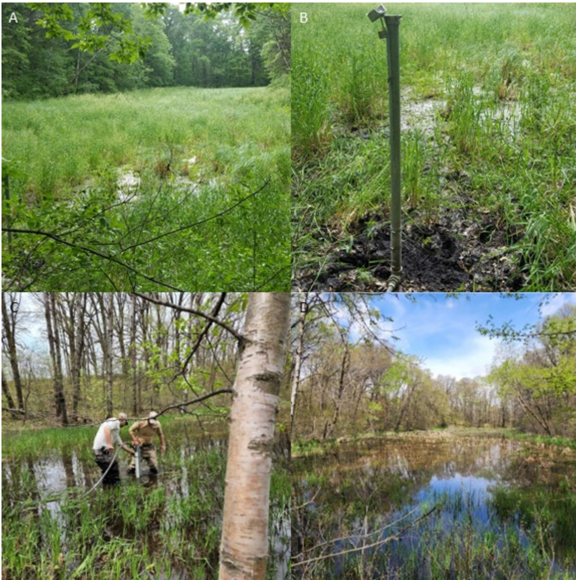
Figure A36: (A) A view of Grey Eagle WMA 2 (note well in lower left corner) on June 9, 2020. (B) Steel casing housing bubbler orifice line, taken on June 9, 2020. (C) Installation of OTT equipment on May 18, 2022. (D) A view of Grey Eagle WMA 2 with inundation on May 18, 2022.
