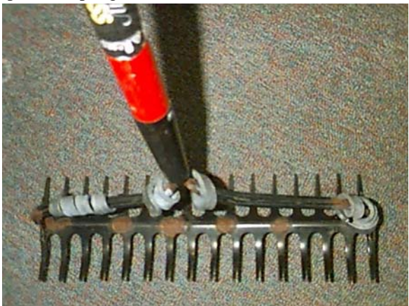
Double-headed garden rake used for submerged plant sampling.
