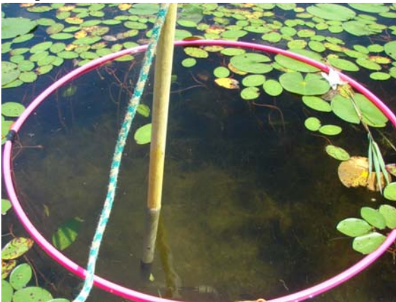
Plastic hoop (one-meter squared area) to delineate sample area.
