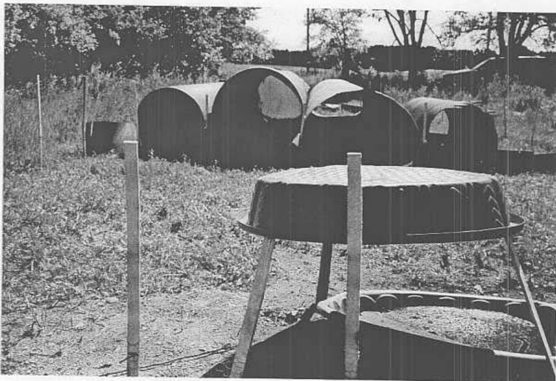
Figure 16. (above) Culvert array (left to right: 36" rd, 48" rd, 48" sq, 36" rd) view looking east in direction of travel to nesting dunes, visible as distant treeline. Plank gates limited access; note tarp covering far end of 48" rd vs. open 48" sq.
