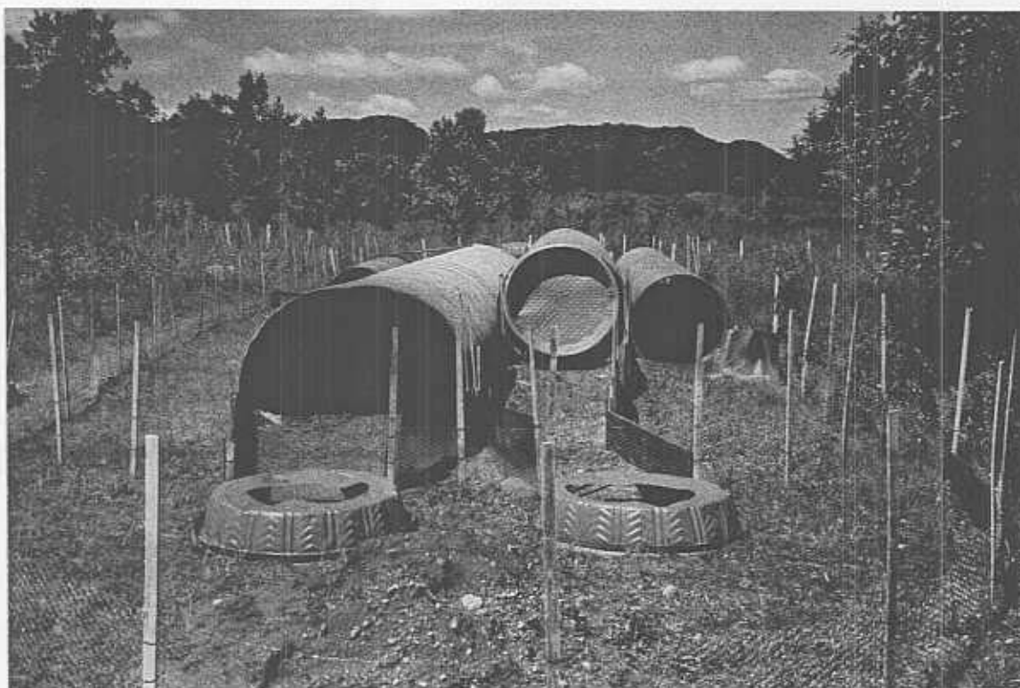
Figure 17. (below) Test culverts, looking west, showing traps and runways so culverts could be tested in different combinations. Plastic covers end of 48" rd. Culverts shown are: (right to left) 48" squashed, 48" round, and 36" round.
