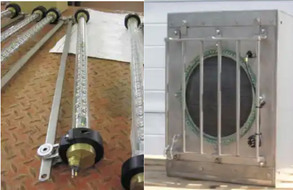
Figure 6-2. Example of the FGS MkIII 30–600 Hz Sound Projectors and High-Intensity LED Strobe Light Bars. (Accessed 2025 DEC 07; Photo credit: Turnpenny 2016)
