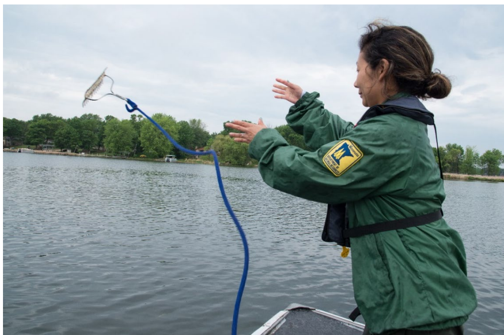
Figure 2. Throwing the sampling rake.
