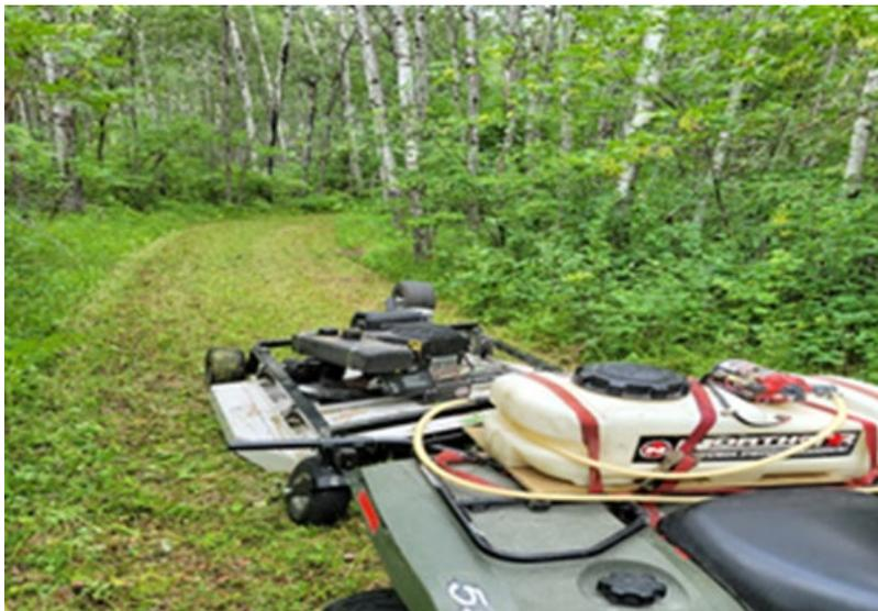
*A brush mower pulled behind a four-wheeler is used to mow Hunter Walking Trails late each summer.*
