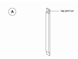
Cut three of the 12 foot 2x4 into two 4 foot long pieces, then cut a 3/4" deep and 3 1/2" wide section out of each end for a total of 24 lap cuts
