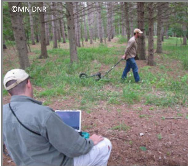
Ground penetrating radar detects anomalies, or differences in soil composition, such as would be made by compaction, excavation or other disturbances.
