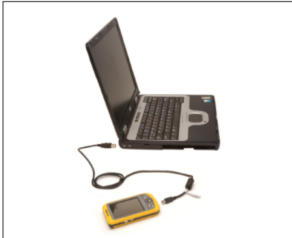
Figure 4.1 Connecting the handheld to a computer using the USB data cable
