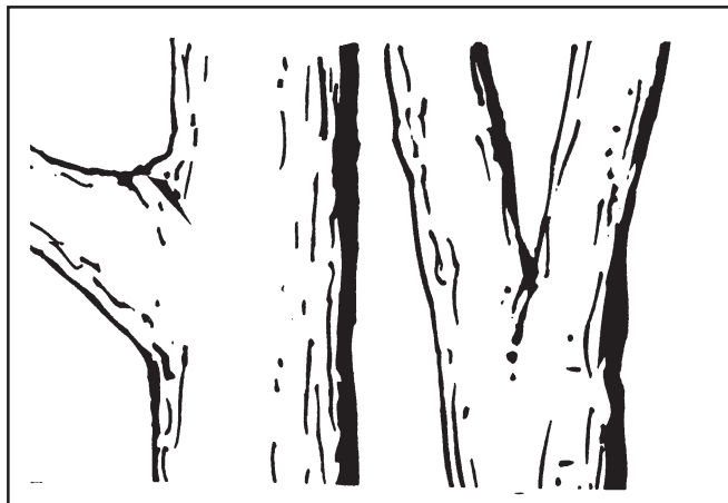
Figure 10: Types of branch unions U-shaped strong union (left) and V-shaped weak union (right)
