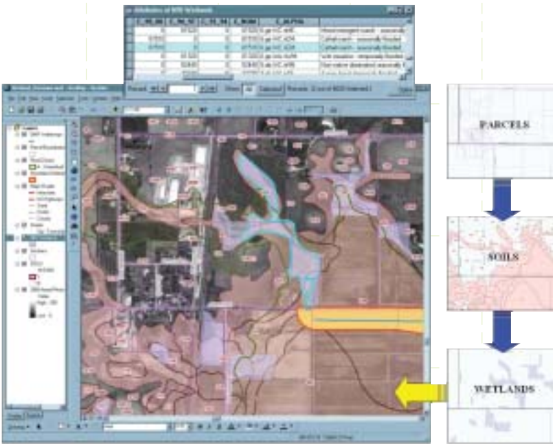
FIGURE 3: MAPS IN A GIS CAN BE OVERLAPPED AND LINKED TO A DATABASE.
