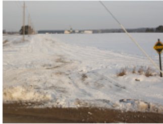
Although this crossing is well marked from both sides, it is not optimal due to the guy wire from an adjoining utility pole. During the day, riders are likely to see it, but at night it poses more of a risk. Careful attention to detail is essential at all crossings given the distractions that are inherent in these situations.
