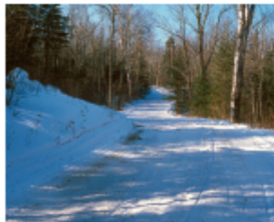
Larger, flowing curves with adequate sightlines are preferred for snowmobile trails. Sightlines should be long enough for the rider to react to oncoming conditions but not so long as to entice excessive speeds.
