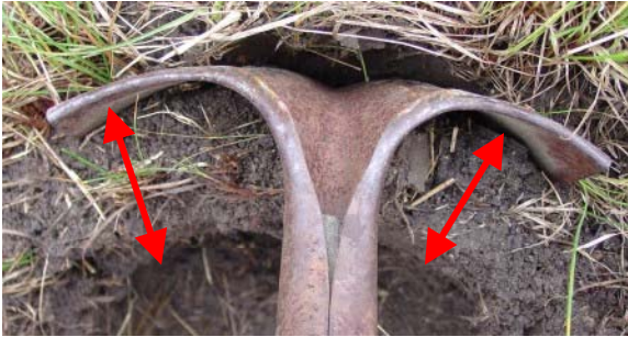
Photo 2. Keep the width of the soil slice uniform along the entire 6 inches
