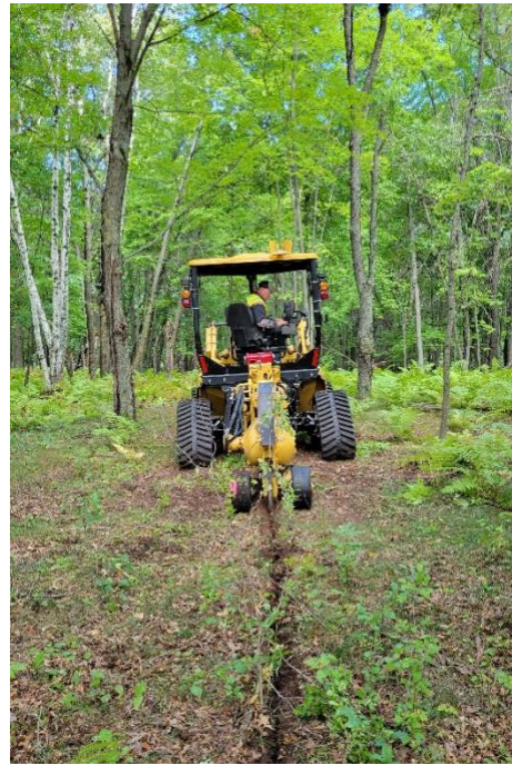
Figure 4. A vibratory plow severing roots, making a barrier line.
