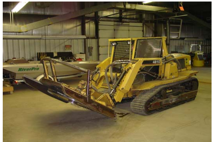
Mower or grader blades striking rocks can cause sparks that start fires.
