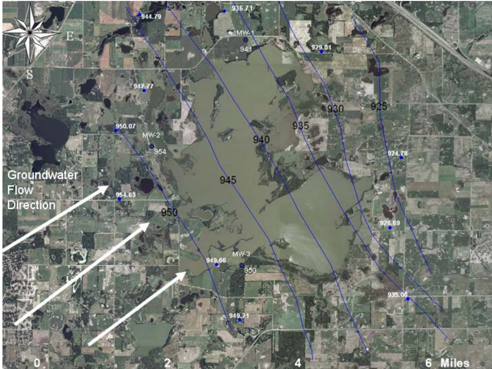
Figure III.B-3 Regional Quaternary Groundwater Contours and Flow Direction
