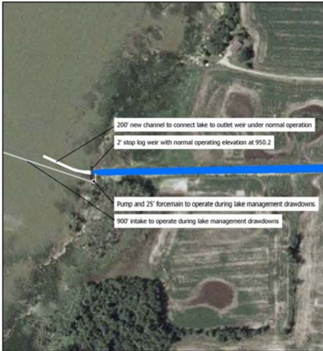
Figure V.B-1 Lake Outlet Controls
