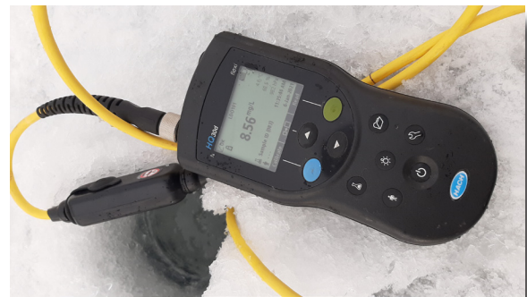
ABOVE: A dissolved oxygen meter in action. The meter is reading 8.56 milligrams of oxygen per liter of water - a comfortable level for all local fish species.
