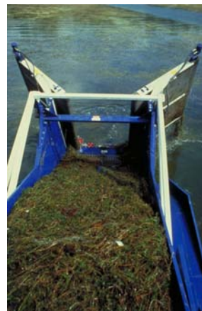
A mechanical harvester cuts nuisance mats of curly-leaf pondweed on a lake.
