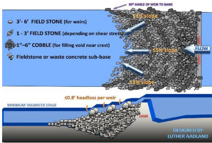
Schematic of a typical rock arch rapids that would allow fish to swim upstream past the dam.
