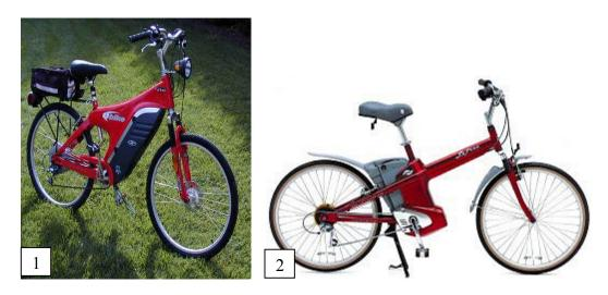
These devices are only a sampling of what is on the market. On average, they can operate at speeds of 13-20 miles per hour. The bicycles can be pedaled faster than 20 miles per hour but the motor assistance will stop after the bike exceeds 20 miles per hour. However, not all electric bicycles operate within these parameters. The rider's weight, terrain, and battery charge are factors in the bicycle's overall speed.
