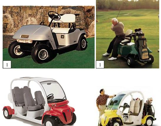
Electric golf carts vary in length and width and there are many available models. The model shown (upper left) has an average speed of 12-14 miles per hour. However, the speed is dependent on terrain, rider's weight, and battery charge. Due to the variability of makes and models, not all types can be shown.
