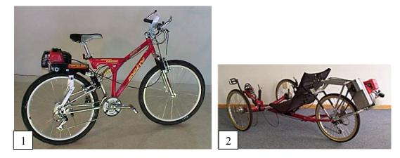
These devices are only a sampling of what is on the market. These bicycles can travel up to 30 miles per hour. The speed is dependent on the rider's weight, terrain, and the size of the engine that is mounted on the bicycle.
