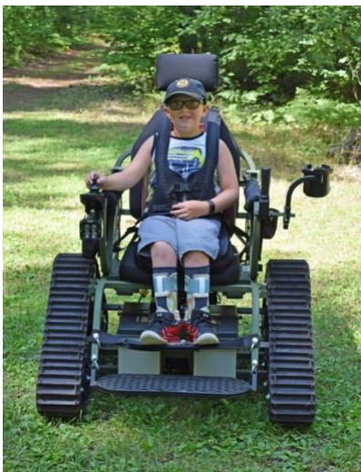
Figure 5. Track chairs are specialized mobility devices equipped with tracks instead of wheels, allowing users to explore rugged terrain and natural surfaces.
