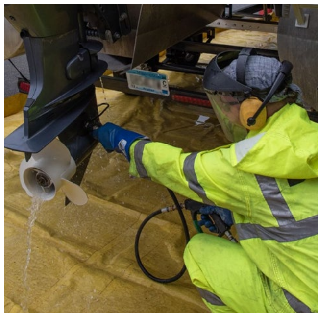
Level 2 Inspector Matt Dwelly conducts an engine decontamination on a pontoon boat's outboard motor in 2022.
