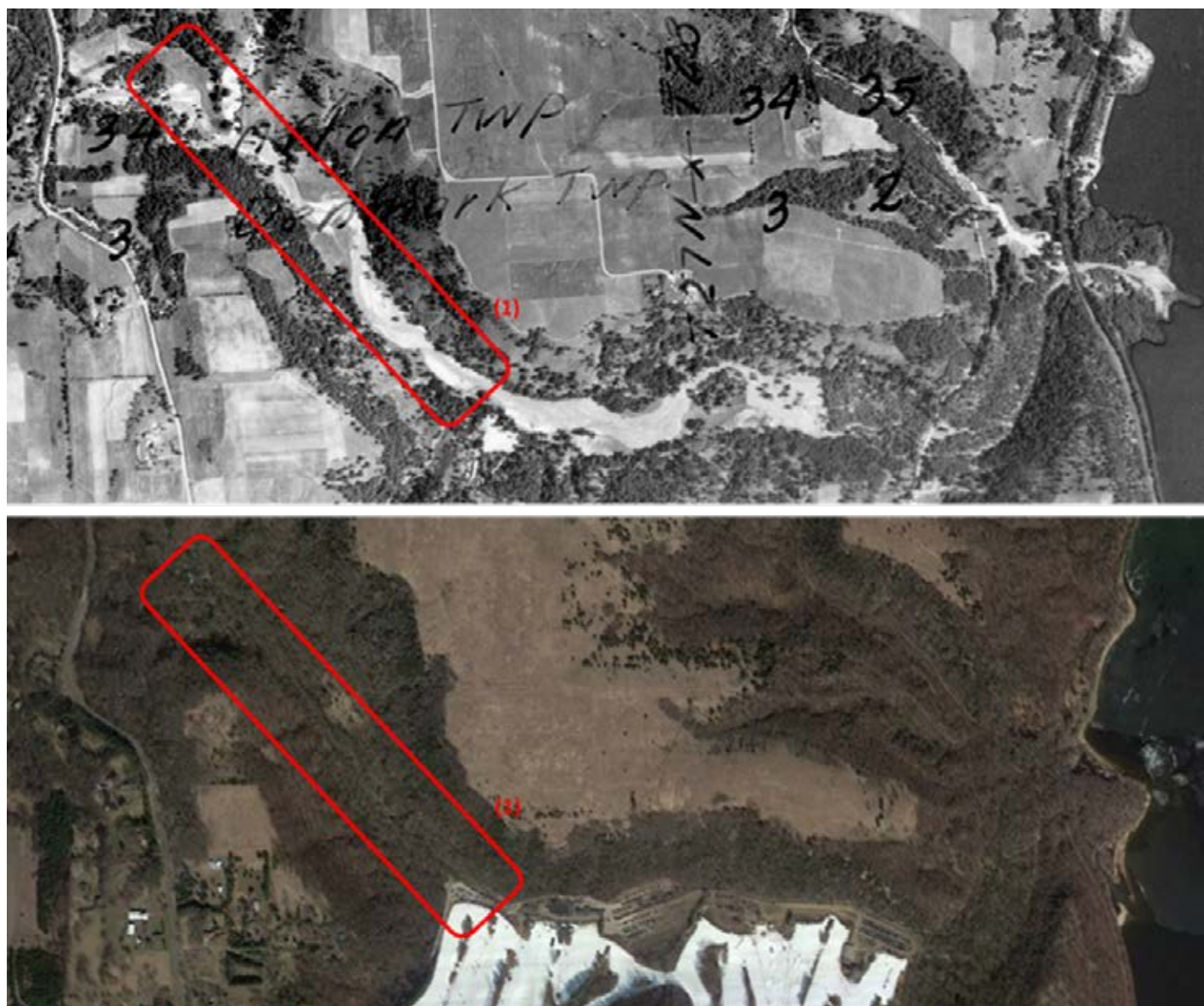
Figure 39-2 Aerial Photo comparison of 1938 imagery (upper) and 2016 imagery (lower). Note lateral instability and aggradation of project area (1) apparent 1938 photograph.
