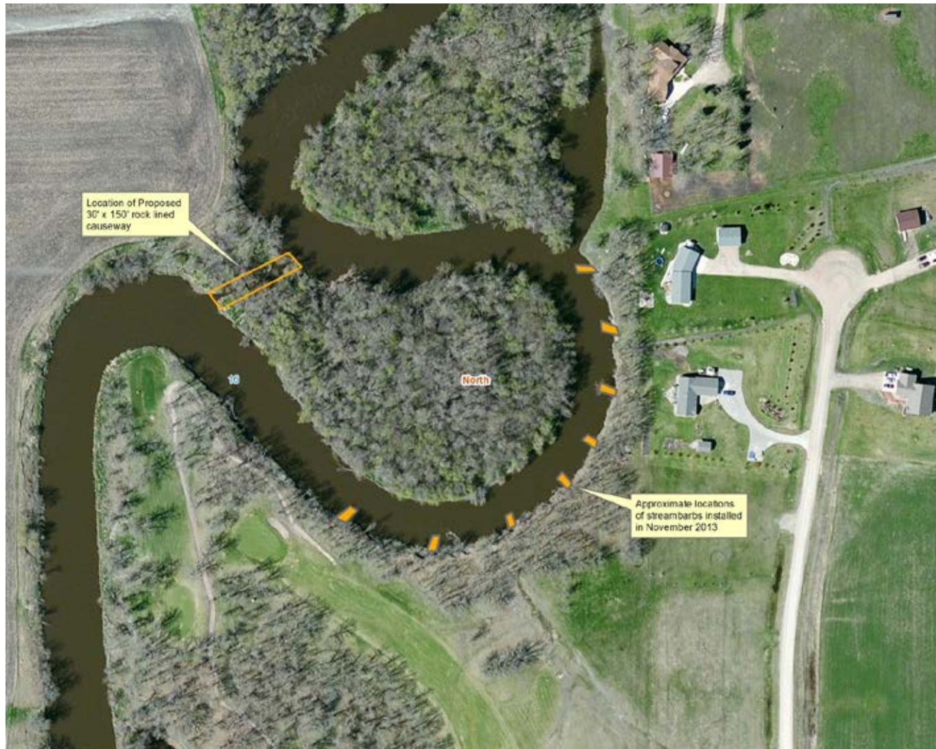
Figure 11-1 Map of project site on Thief River Meander upstream of Thief River Falls. Locations of installed stream barbs are shown.
