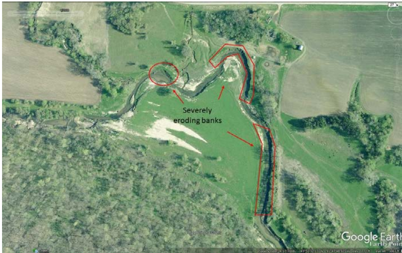
Photo 29-2 Aerial image of the project site from 2008, prior to construction in 2011. Areas highlighted in red indicate severely eroding banks. Aerial photography is from April 2008 and provided by Google Earth.
