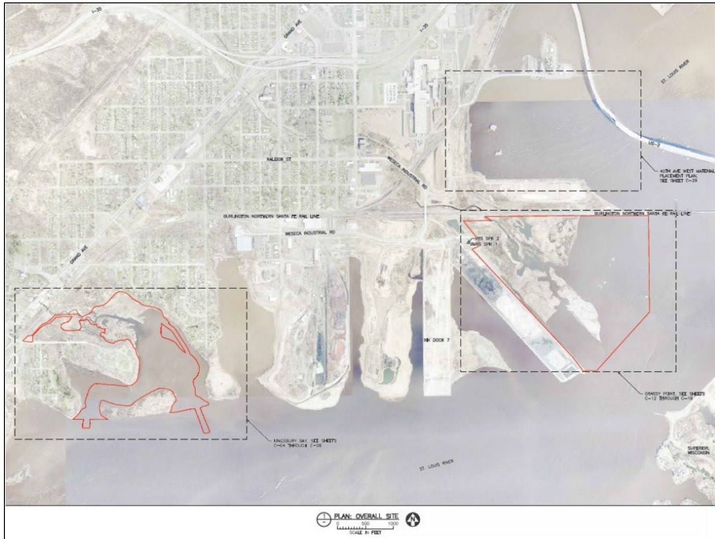
Figure 9. Aerial map of pre-construction conditions for Kingsbury Bay in the red box along the left hand side of the map and Grassy Point in the red box along the right hand side of the map. Dredged material from Kingsbury Bay was taken to Grassy Point and used as biomedium to improve aquatic and terrestrial vegetation growth post-restoration.
