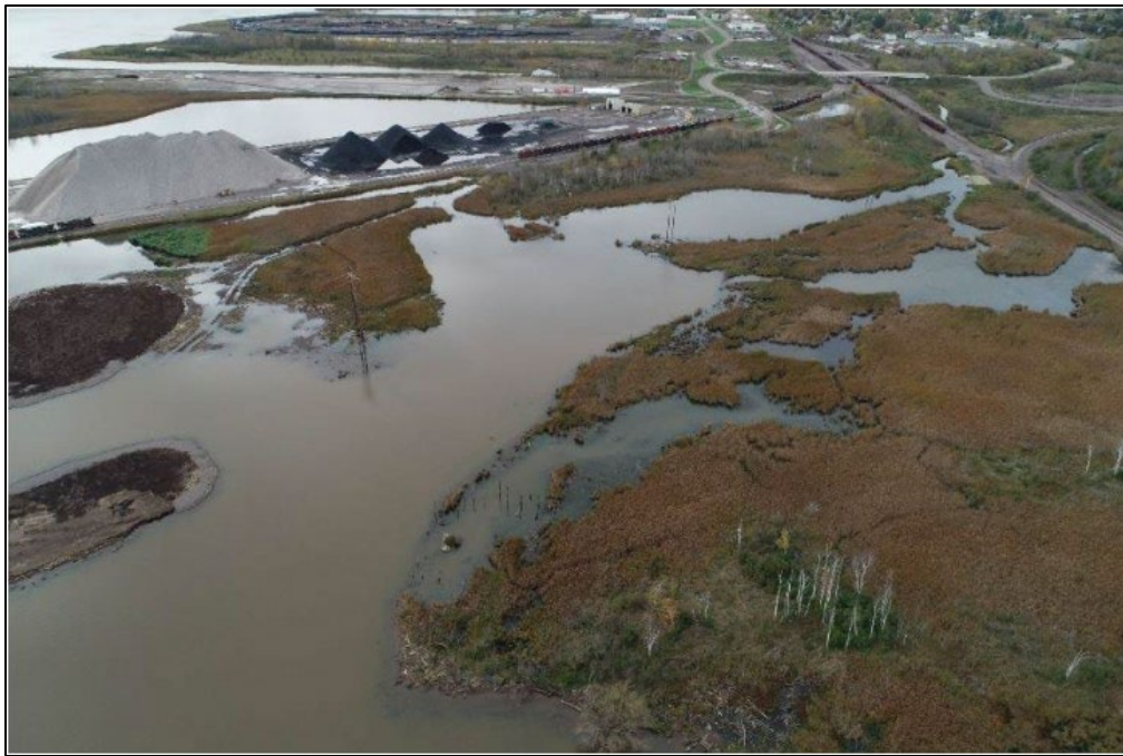
Photo 7. Aerial view of the interior of the Grassy Point wetland complex where legacy wood waste was removed to create deeper water depths more similar to historic and reference conditions. The mouth of Keene Creek in the upper right hand corner of the photo was dredged to increase water flow through the wetland. Photo provided by MNDNR Lake Superior and St. Louis River Program.
