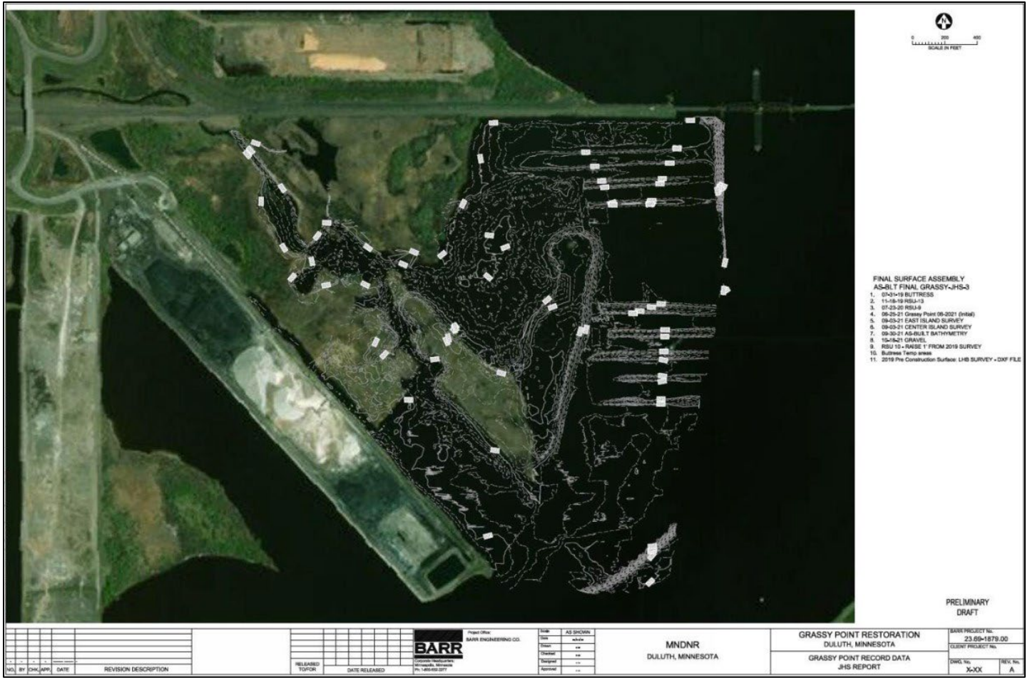
Figure 3. As-built condition contours for Grassy Point following restoration. (Contours were overlaid on an aerial photo taken from prior to restoration).
