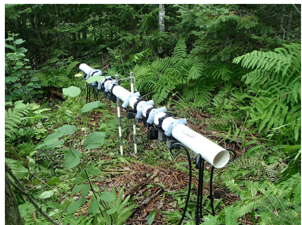
Figure 2. Polyvinyl chloride (PVC) pipe bounce-test structure used to quantify environmental and animal movement effects on expansion of Global Positioning System (GPS) collar bands, 2014 to 2015, in northeastern Minnesota and St. Paul, USA. The PVC pipe was 10.2 cm in diameter, resting on 2 metal stands, each 54 cm tall.
