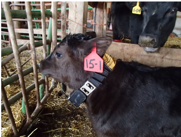
Figure 3. A 12-day-old Angus beef calf collared with the 2015.2 generation collar on 30 March 2015 in Scandia, Minnesota, USA. The collar was removed by the owner 332 days postcapture.
