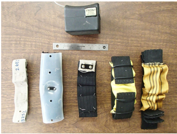
Figure 1. GPS PLUS VERTEX Survey-1 GLOBALSTAR package (top) and expandable bands (bottom: left to right): 2013, 2014.1, 2014.2, 2015.1, and 2015.2, deployed and tested 2013–2015, in Minnesota, USA.
