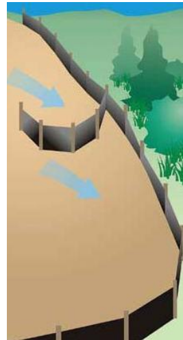
"J-hooked" silt fencing
