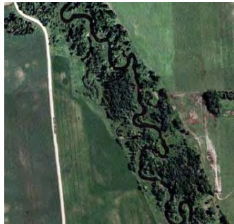
(above) Buffered : The vegetated buffer along the Pelican River decreases the contaminants and sediment carried by runoff to the stream.
