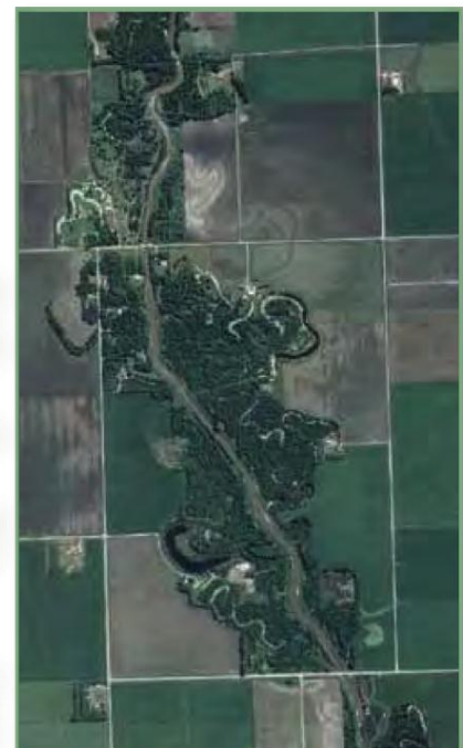
Land use change and channelization: The floodplain and stream corridor are impinged by agricultural fields. The meanders are disconnected after straightening by channelization.
